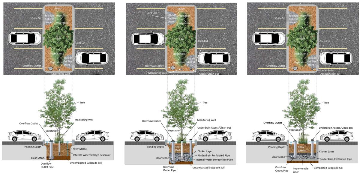
Stormwater planter / Bioretention - No infiltration
