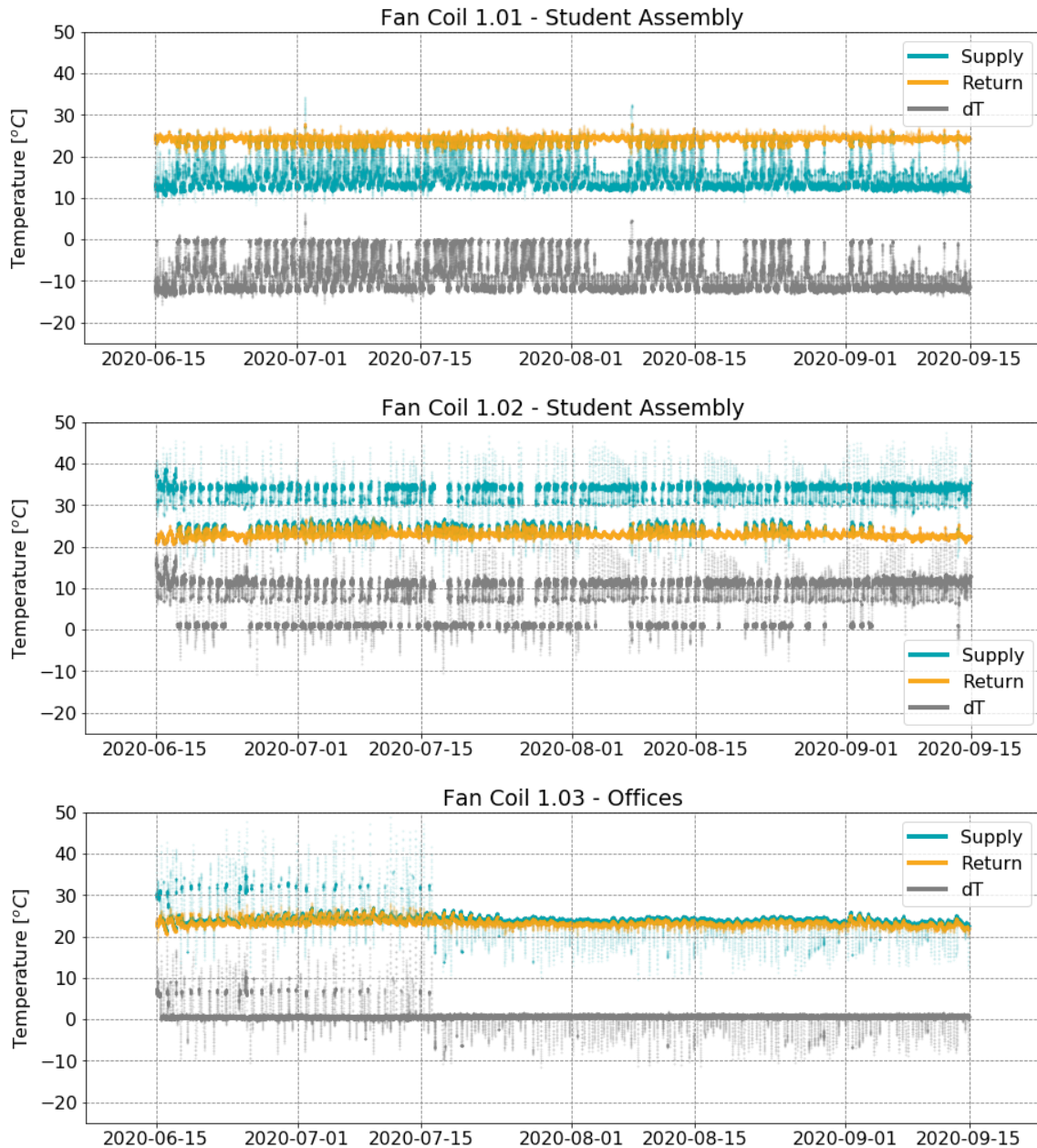
Figure 7-1. Supply and return temperature (and their difference) is shown for Fan Coils 1.01, 1.02, and 1.03.
