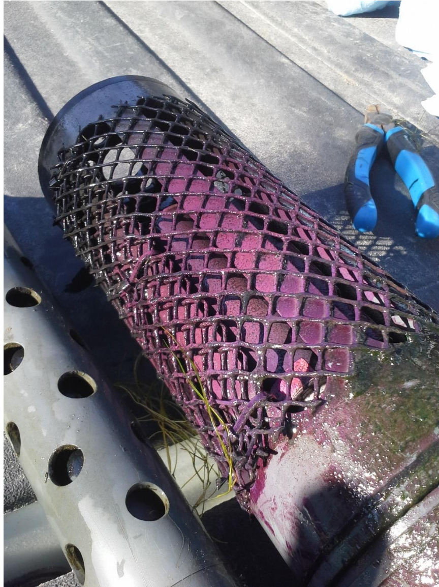
Figure 41. Purple-sulphur bacteria, and extremophile, colonizing a water quality sonde at Site C Pond, June 20, 2016.
