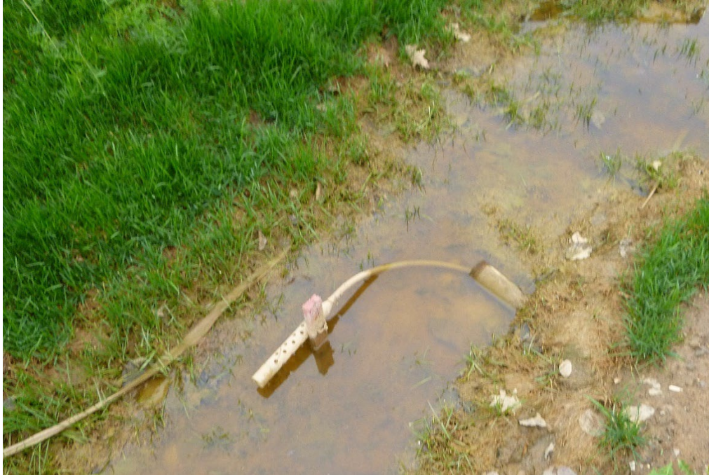
Figure D1: Installation of sampler intake in swale, the pipe that can be seen in the bank of the swale leads back to the equipment box.
