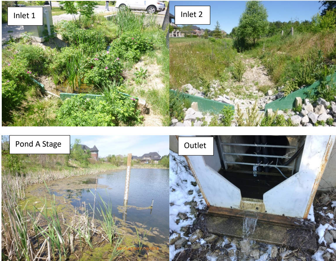
Figure 6: Monitoring infrastructure at Pond A. Note: Stage is located in aftbay of pond and is viewed from the outlet structure in photograph.
