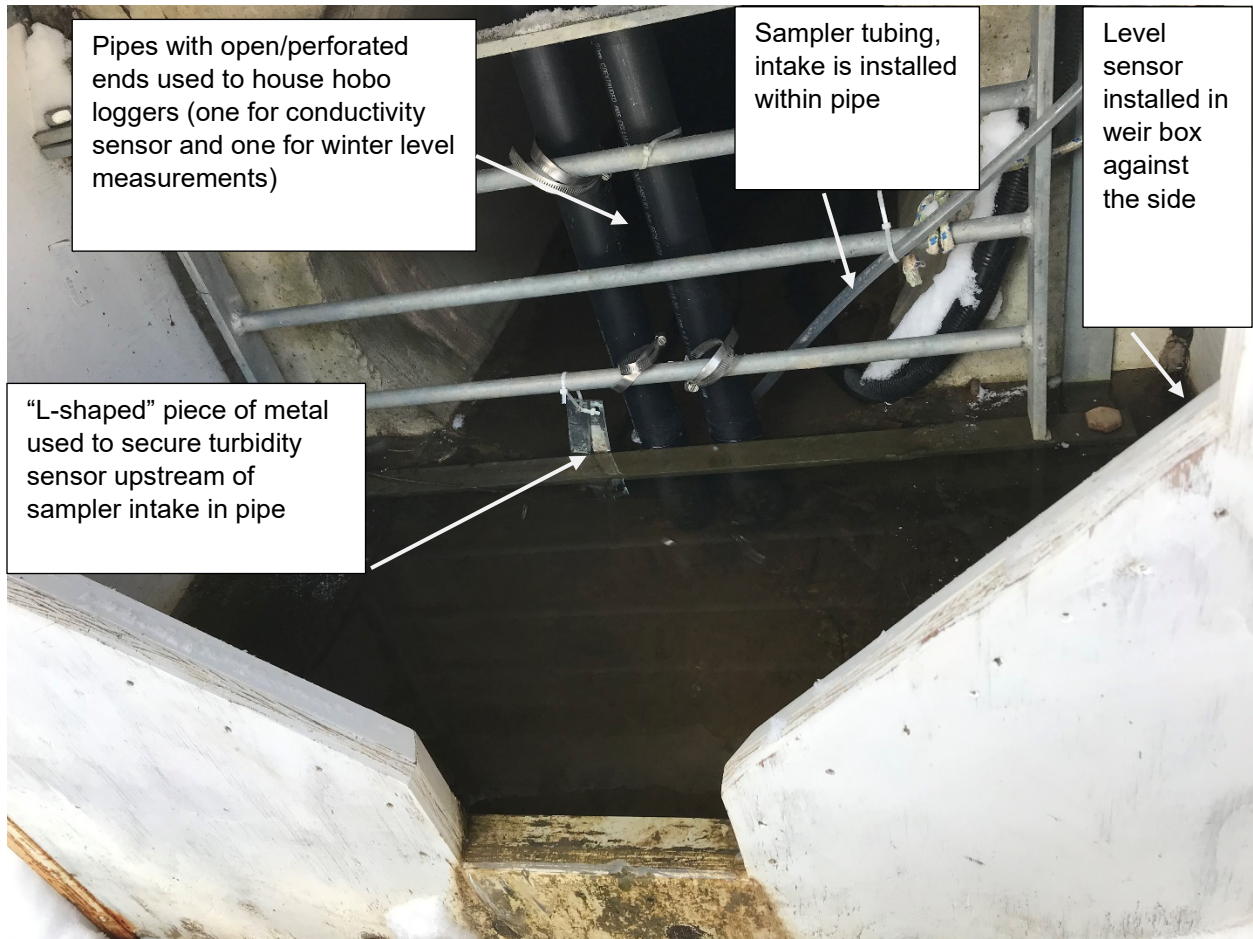
Figure D4: Outlet monitoring station layout.
