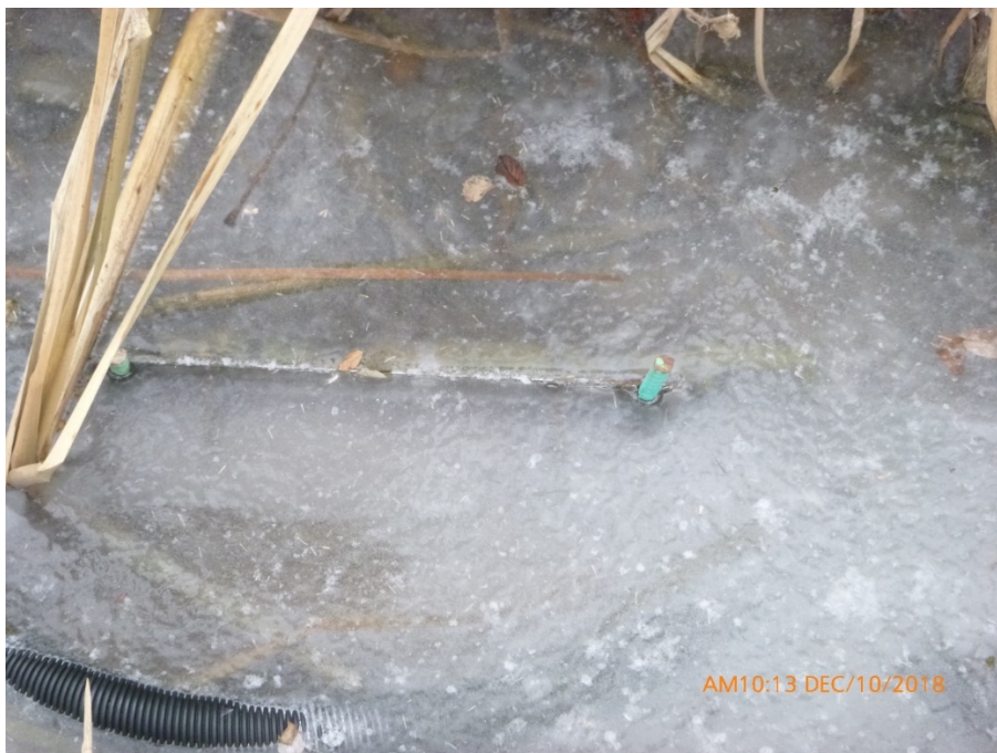
Figure D9: Turbidity sensors were left in place during the winter to capture melt events. However, the wiper was removed to prevent the motor burning out when it got stuck in ice.
