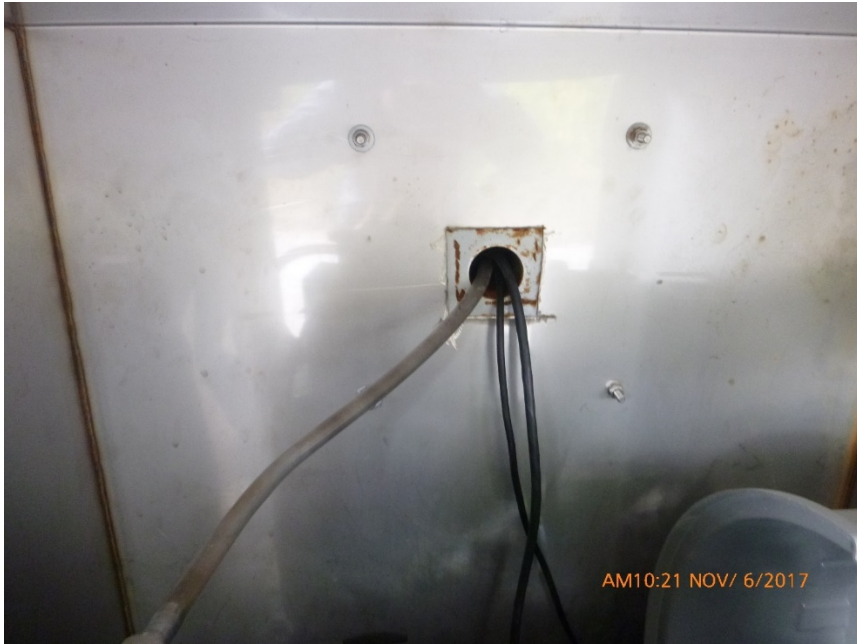
Figure D3: Illustrates port through which the tubing and sensor cables are directed out of the sampler box.
