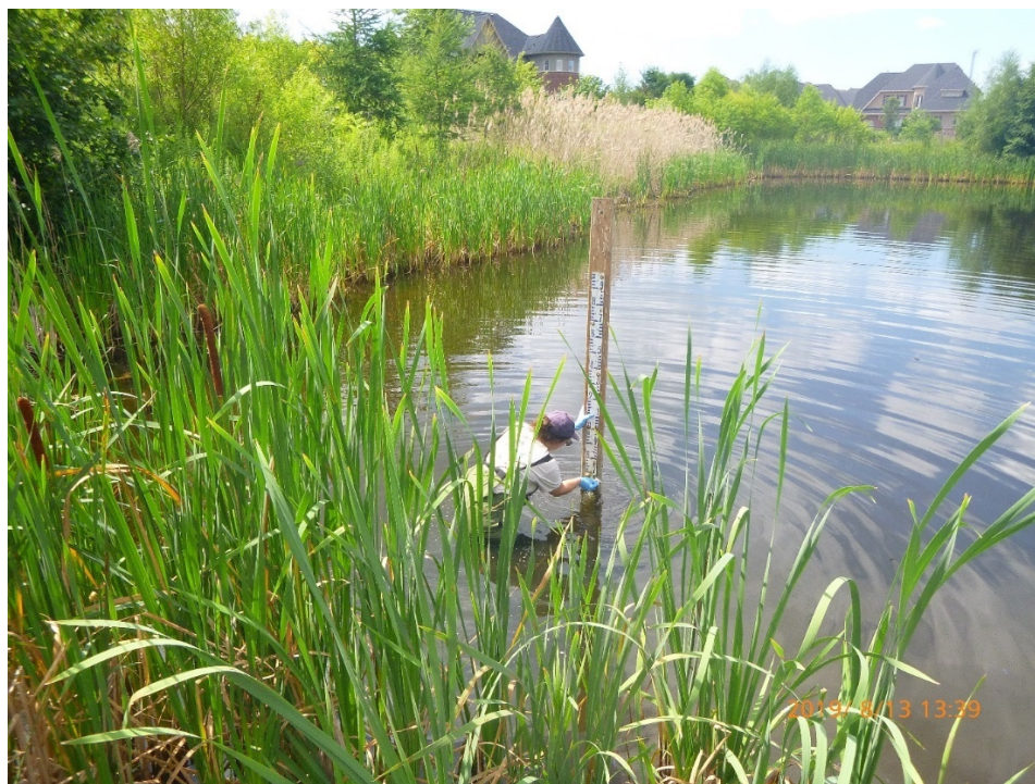
Figure D7: Illustrates staff gauge cleaning that was required after 2 years due to algae build up that made the stage unreadable.
