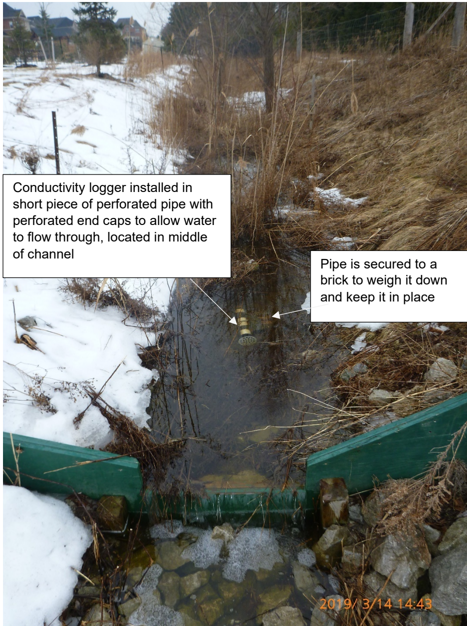
Figure D5: Shows how conductivity logger is installed in inlet swale.
