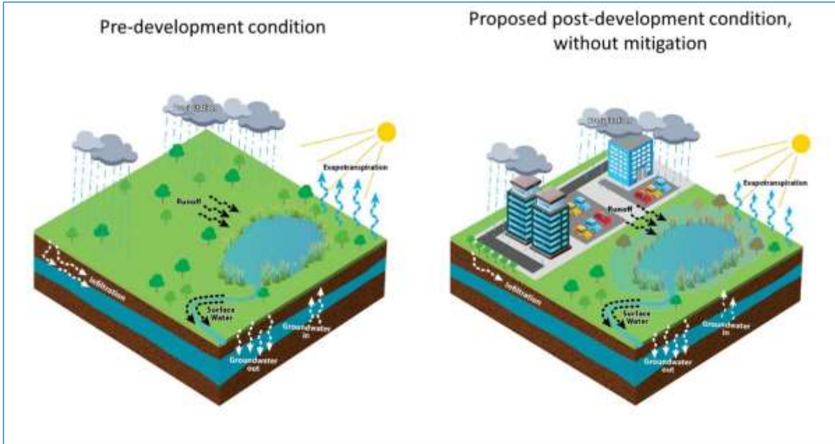
Figure 15: Development increased runoff volume to the wetland and reduced infiltration
