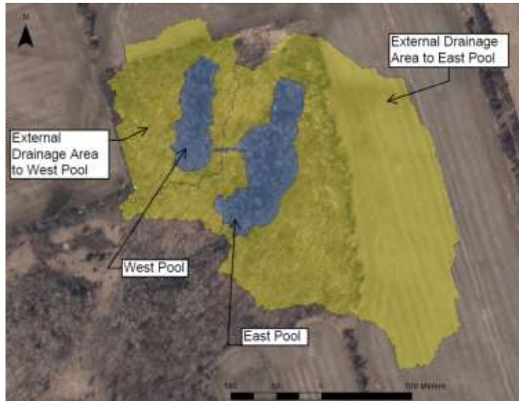
Figure 5: Example of wetland with two distinct hydrological units or pools
