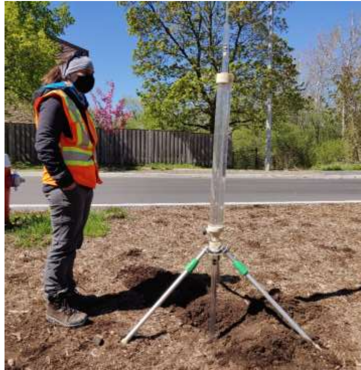
Topsoil infiltration exceeds design rate (30 mm/hr)
