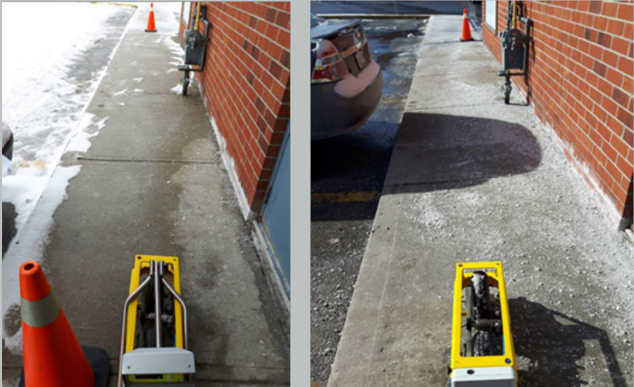
Figure 2: Friction values for a properly treated surface \mu = 0.63 (left image) and an oversalted surface \mu = 0.26 (right image)
