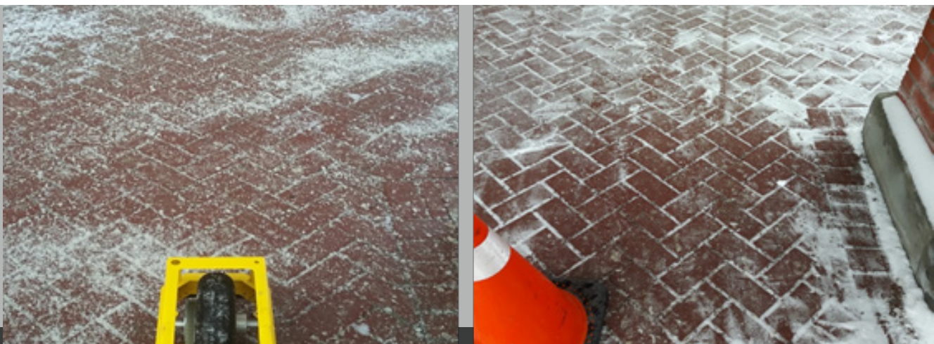
Figure 3: Similar \mu values were measured for an oversalted walkway (left image), and the same walkway which has had the snow shoveled off (right image).
