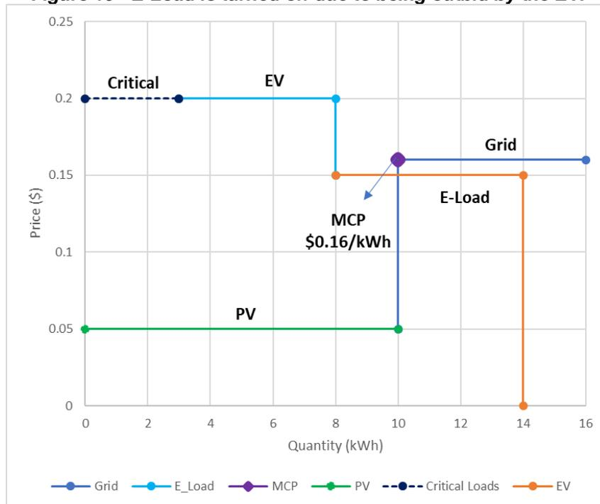
**Figure 20 – Bid #2: Microgrid requires grid import due to high bids from EV and E-Load.**
