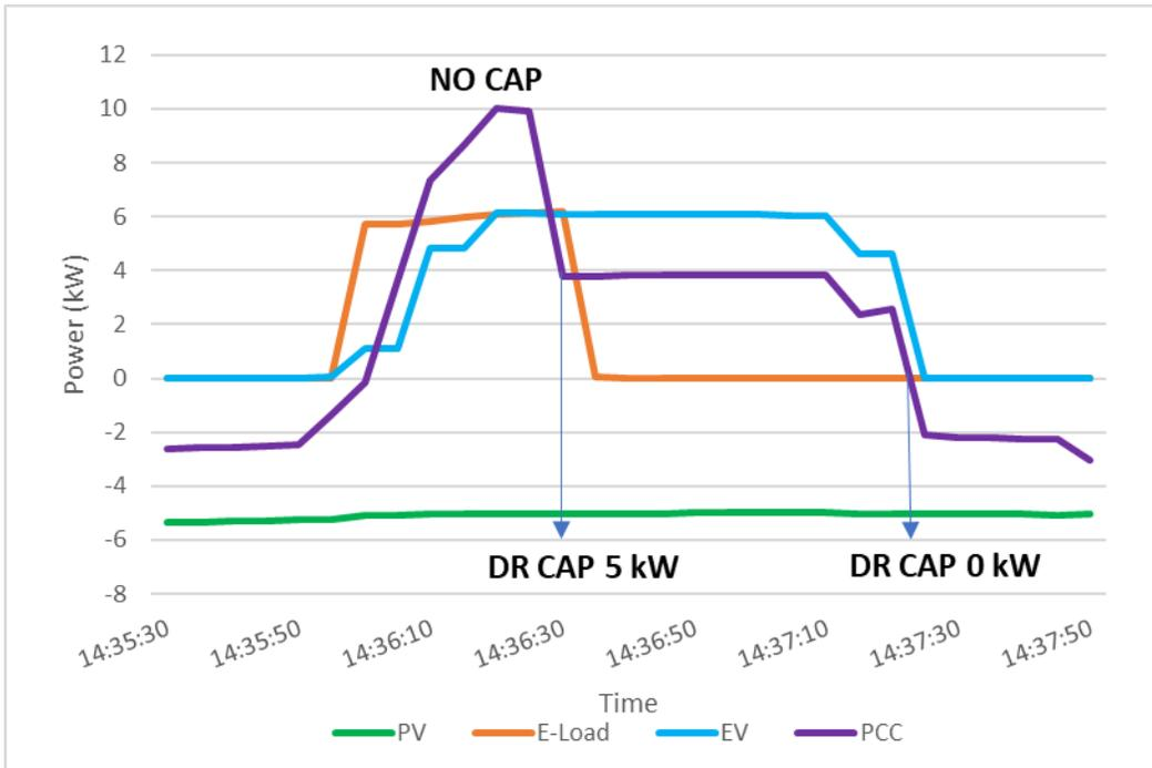
**Figure 22 - Plot of demand response caps altering load profile of microgrid.**
