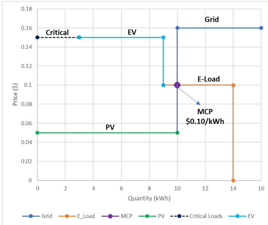
**Figure 19 - E-Load is turned off due to being outbid by the EV.**
