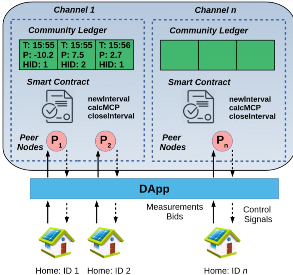
**Figure 7 - Architecture of blockchain-based TEF.**
