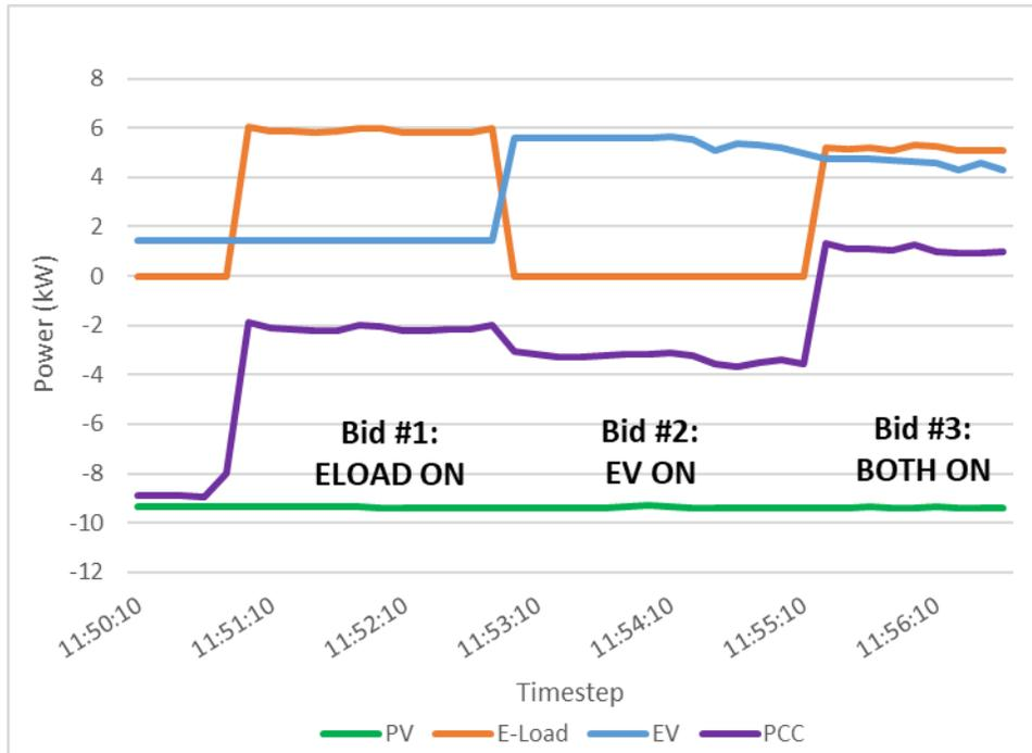
**Figure 21 – Bid #3: Load profile of DERs during all three bids.**
