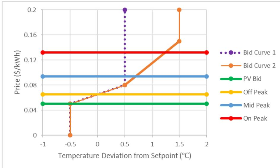
**Figure 4 - Example bid curves of smart thermostats.**
