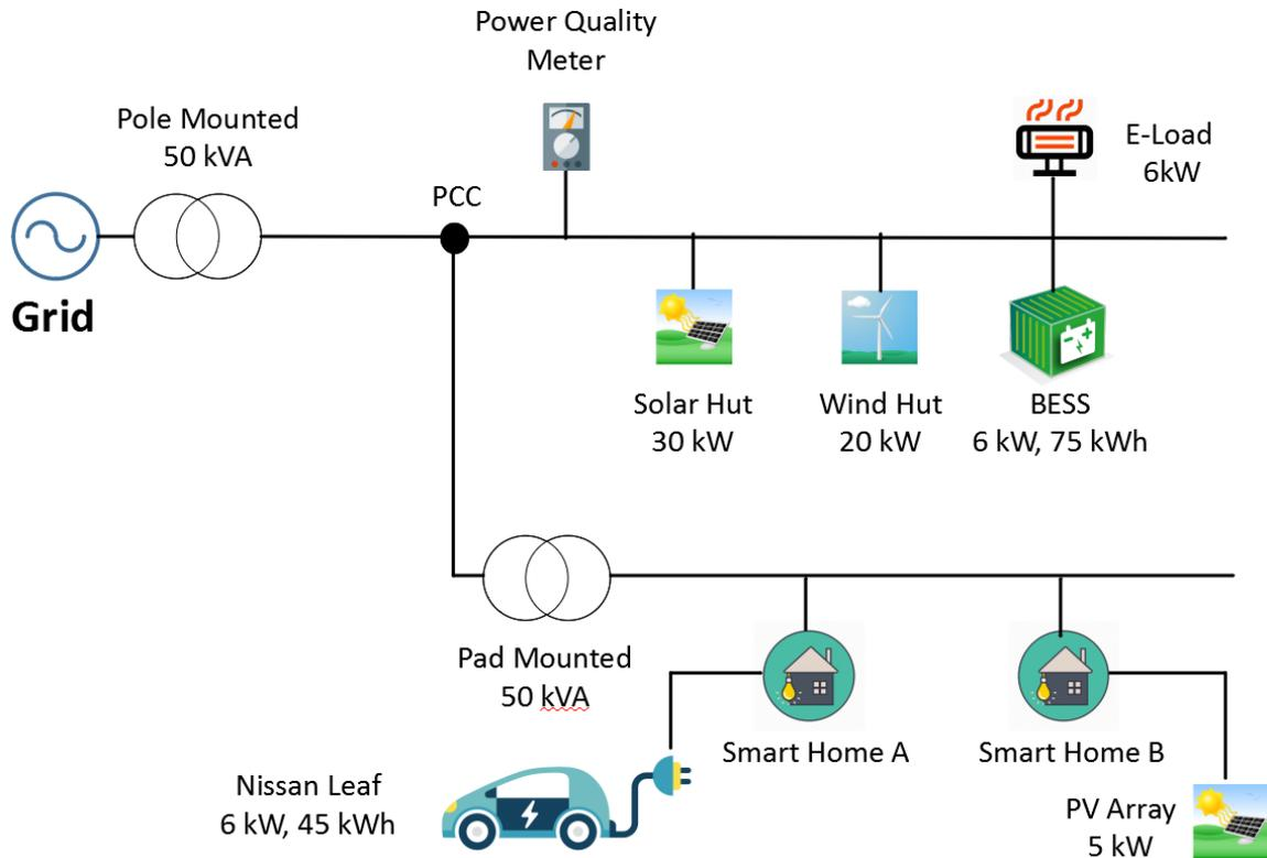
**Figure 8 - Single line diagram of Kortright Centre Microgrid.**
