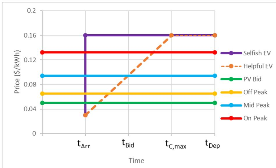
**Figure 5 - Example bid curves of selfish and helpful EVs.**
