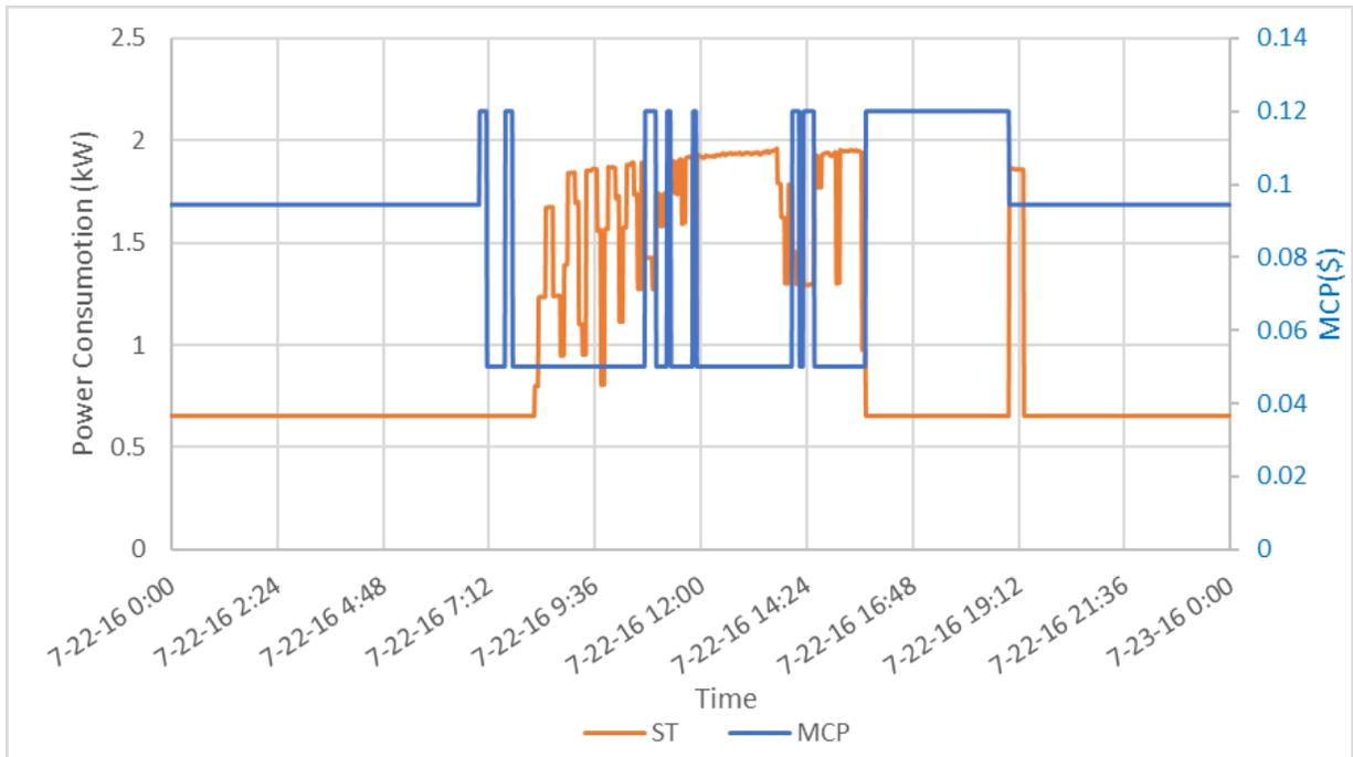
**Figure 12 - Bidding behavior of smart thermostats based on MCP.**
