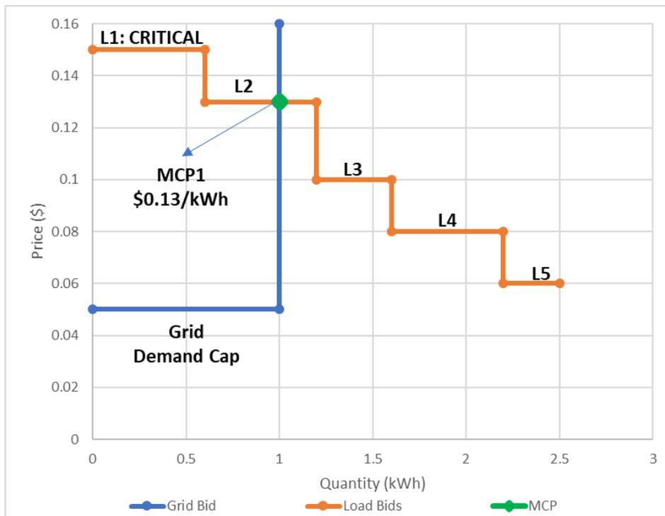
Figure 3 - Vertical grid demand cap limits grid energy supply for the system.
