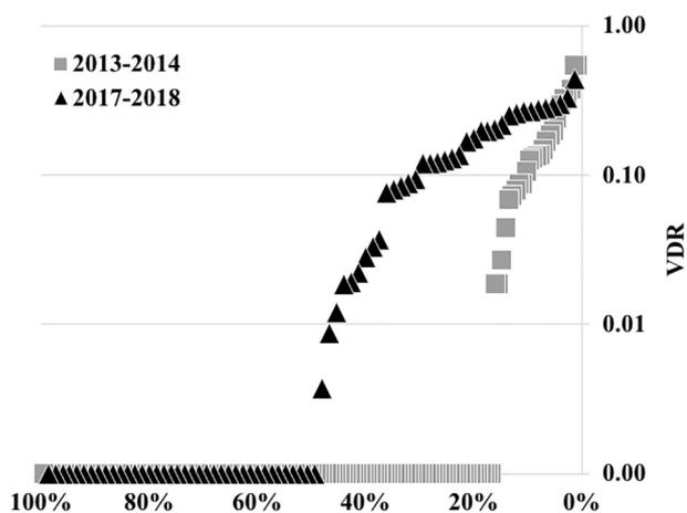
Fig. 3. Cumulative probability plot for Volume Discharge Ratio (VDR, or out-flow volume divided by inflow volume) for the 2013–2014 and 2017–2018 monitoring periods.
