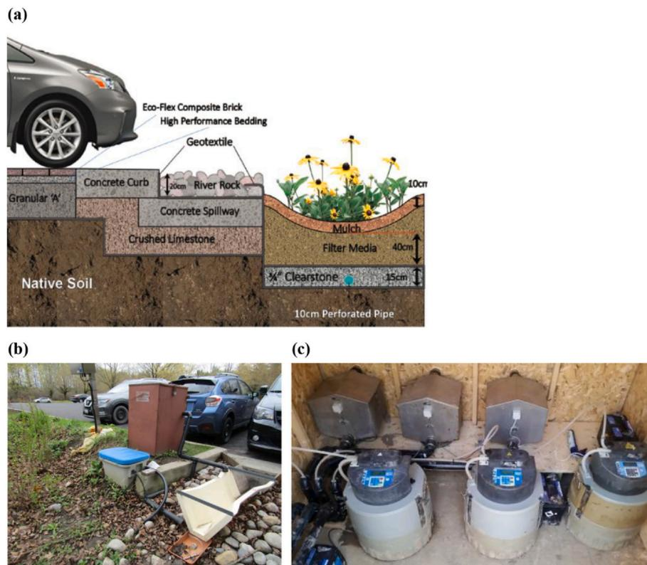
Fig. 1. Site schematic and monitoring equipment. (a) Schematic of bioretention cell (obtained with permission from TRCA STEP (2015)). (b) Inlet monitoring for 2017–2018 monitoring period. (c) Outlet monitoring for both monitoring periods.
