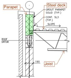
Figure 5 Typical roof assembly
