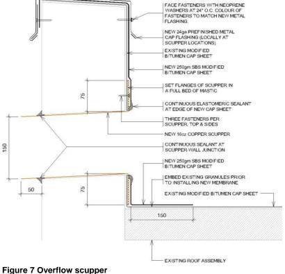
In the case of emergency overflow, the scupper's elevation relative to the roof surface is determined by the roof's maximum load capacity. Once this is calculated, the elevation of the scupper can be determined. Where a roof is flat, an elevation of 19mm (0.75 inches) above the finished roof surface is typical. To allow for main roof drainage, the overflow scupper cannot be lower than the roof surface. See **Figure 7**.
