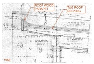
Figure A 1 Steel deck on steel joists, roof without structural parapet
