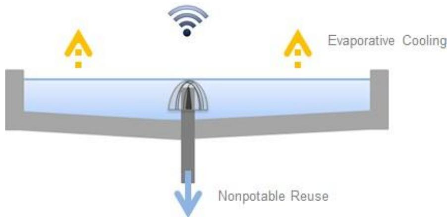
**Figure 2 Graphical representation of concept of an actively controlled smart blue roof system with RWH capacity**
