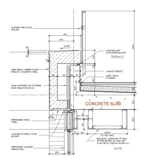
Figure A 5 Hollow Core Precast roof with structural parapet, 2006 Turner Fenton SS, Brampton
