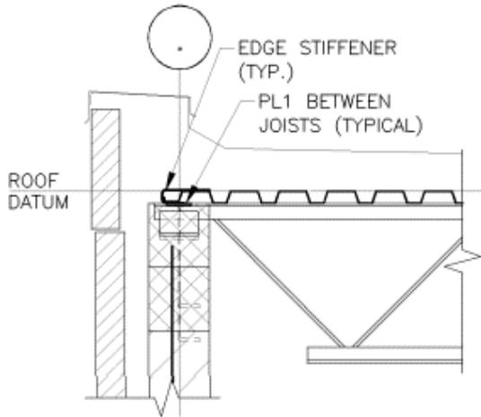
Figure A 1 Steel deck on steel joists, roof without structural parapet
