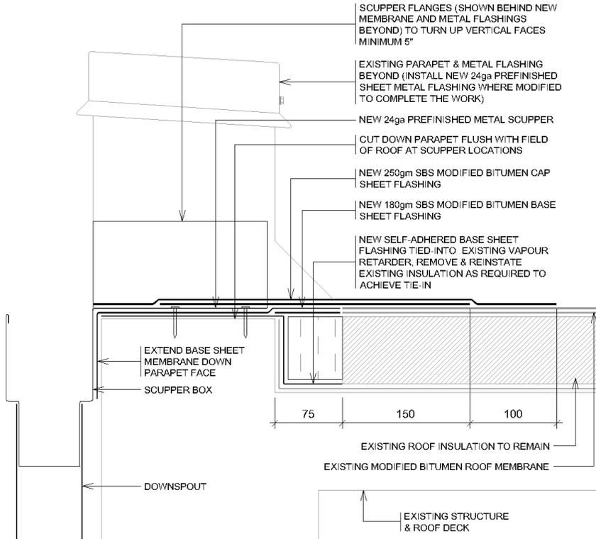
Figure 6 Primary drainage scupper
