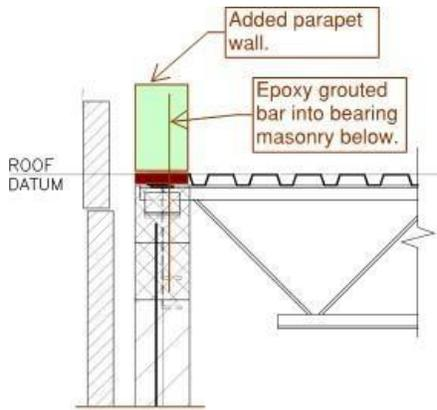
**Figure 8 Adding a parapet wall to bearing masonry**
