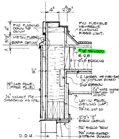
Figure A 4 Plywood on wood joist, roof with structural parapet, 1982 Plum Tree JR. School, Mississauga
