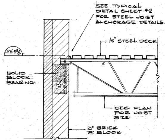
Figure A 3 Steel deck on steel joists, roof with structural parapet, 1974 J.A. Turner SS, Brampton
