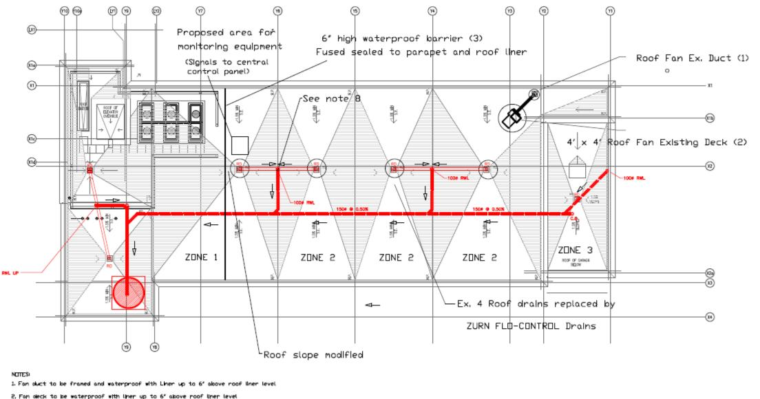
3. Controlled Zones 1 and non-controlled Zone 2 separated by 6' high fixed water proof karrier
