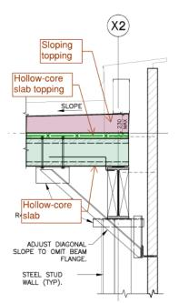
Figure 9 Typical roof structure
