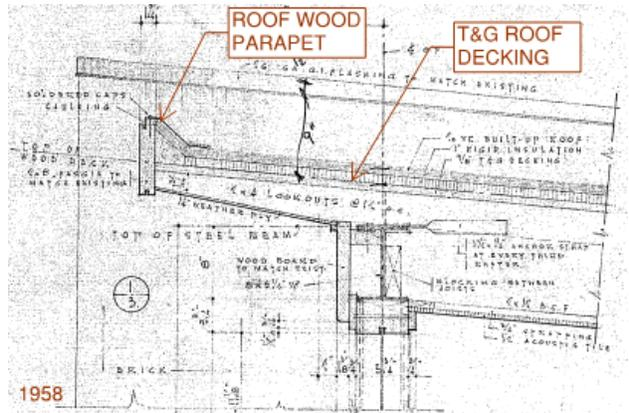
Figure A 2 Roof detail with wood decking, 1958 Kitchener
