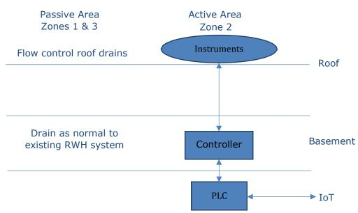
Figure 12 Schematic diagram of Proposed Conceptual Smart Blue Roof with Active Controls and Rainwater Harvesting System
