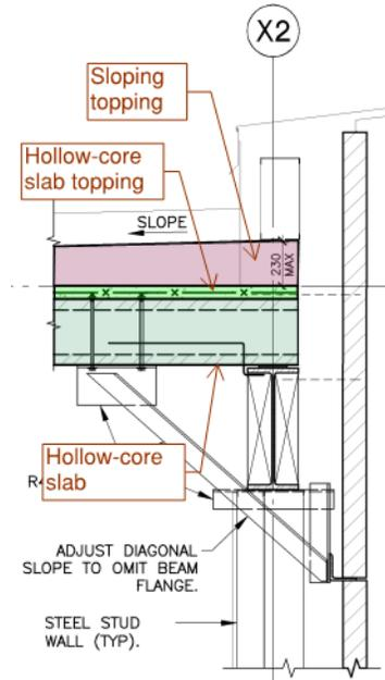
**Figure 9 Typical roof structure**
