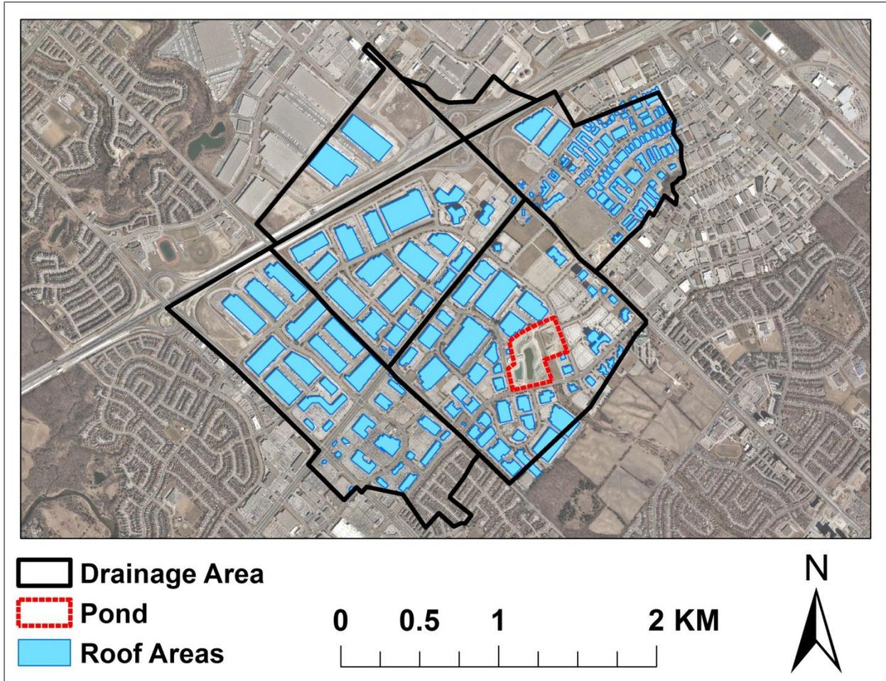
Figure 18 Suitable blue roof retrofit areas within the pond catchment area
