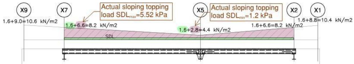
Figure 10 SDL diagram for precast design
