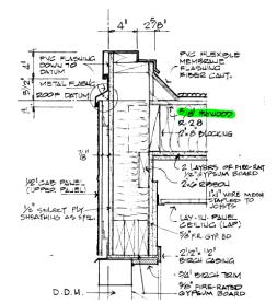
Figure A 4 Plywood on wood joist, roof with structural parapet, 1982 Plum Tree JR. School, Mississauga
