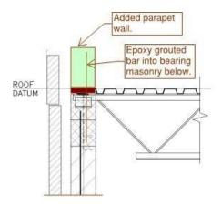
Figure 8 Adding a parapet wall to bearing masonry
