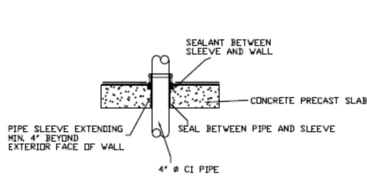
CONCRETE PENETRATION DETAIL (TYP)
