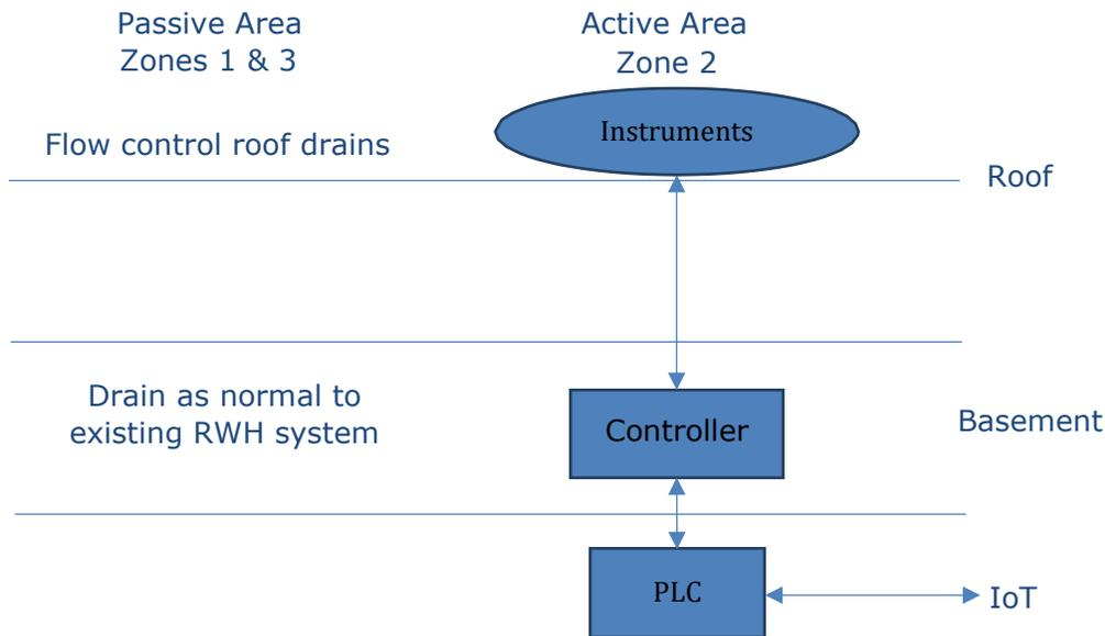
**Figure 12 Schematic diagram of Proposed Conceptual Smart Blue Roof with Active Controls and Rainwater Harvesting System**
