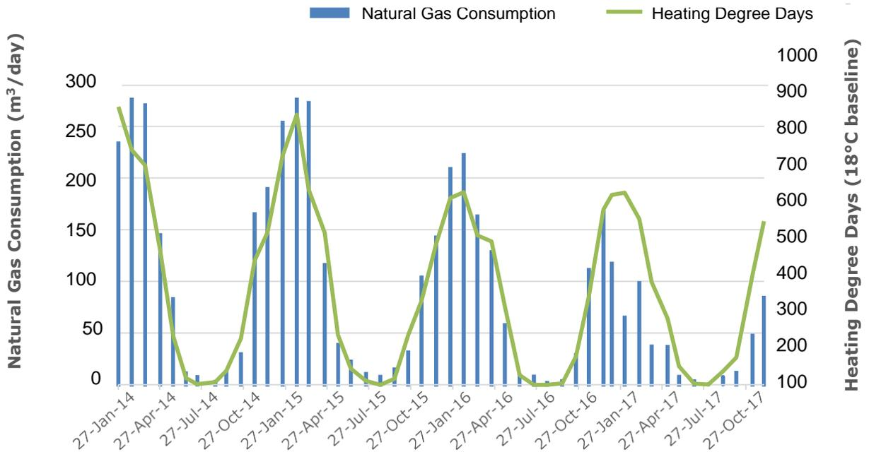
Figure 21 Effects of weather on natural gas consumption
