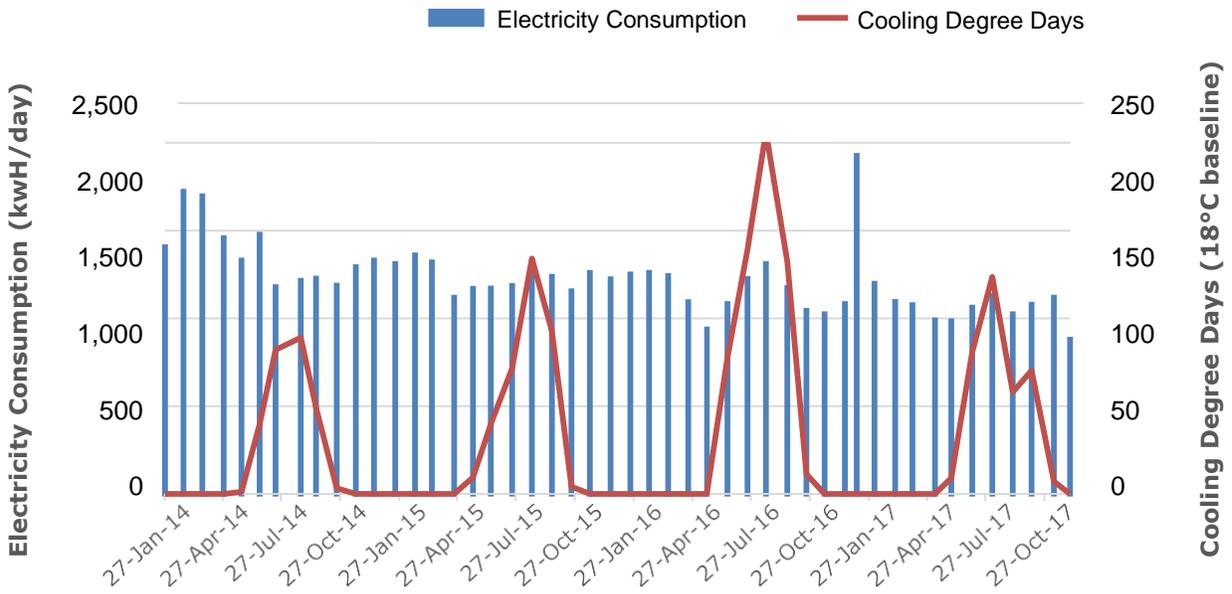
Figure 20 Effects of weather on electricity consumption
