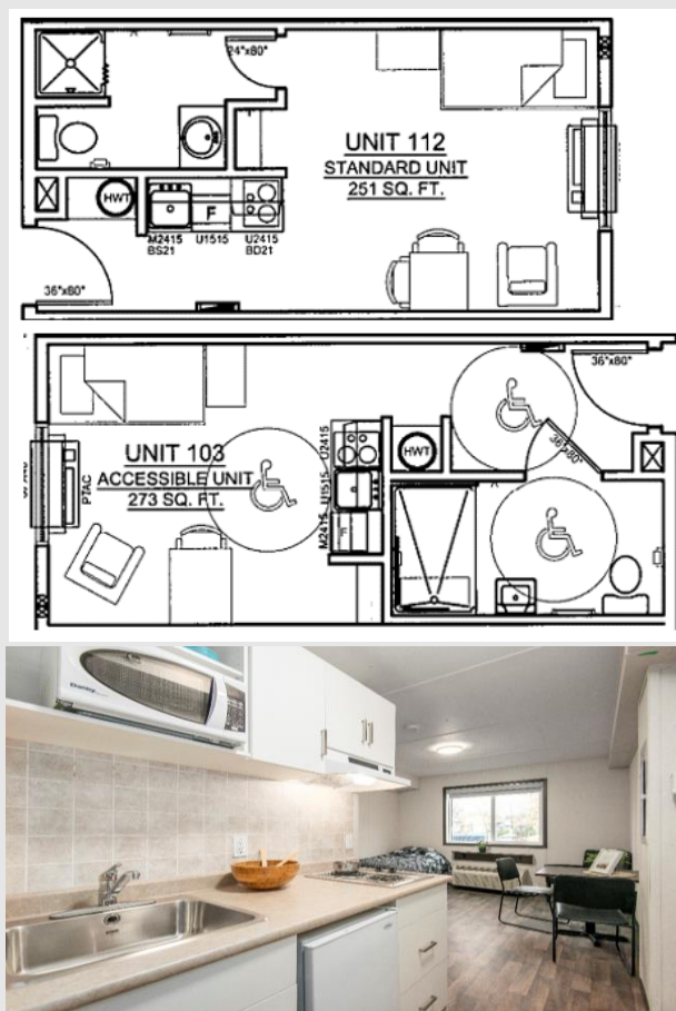
Figure 12. (Top) Example layouts of modular housing units at 220 Terminal Ave. (Bottom) Interior of unit at 220 Terminal Ave. (Credit: Horizon North)
