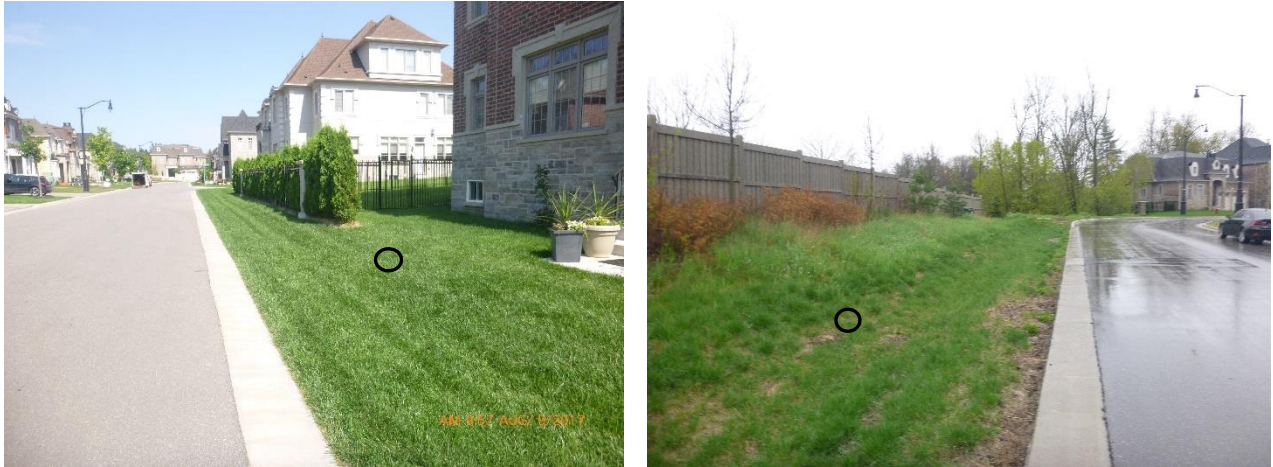
Figure 4-50 and Figure 4-51: Preferred Location for Shallow and Deep Well Installation
