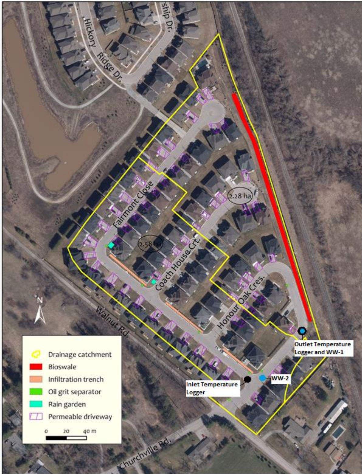
Figure 4-21: Overview of the Wychwood LID subdivision and location of the inlet and outlet temperature loggers as well as the WW-1 and WW-2 monitoring manholes.
