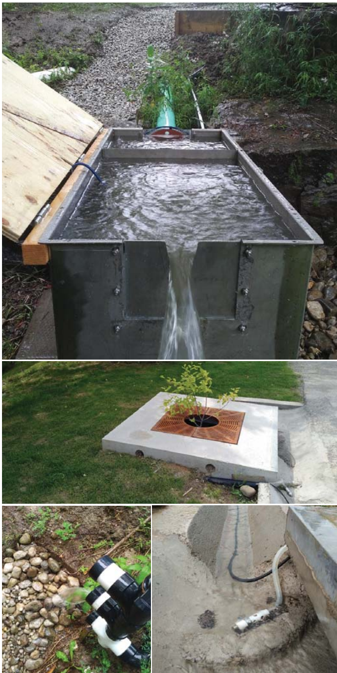
Figure 3. Outlet V-notch weir box (top), service berry shrub (2nd from top), inlet gutter & throat with sampler intake and area velocity probe (bottom right), overflow measurement device (bottom left).
