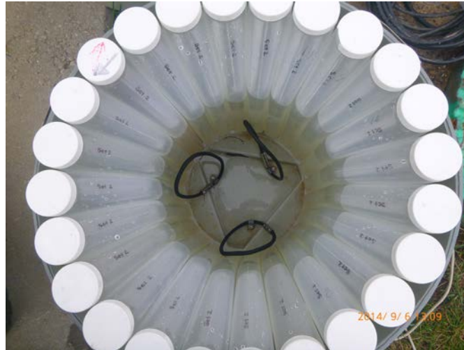
Figure B-1: Example of an automatic sampler base with 24 1-litre sampling bottles
