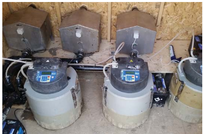
Figure 5. Tipping bucket flow meters and water quality samplers inside the monitoring hut.
