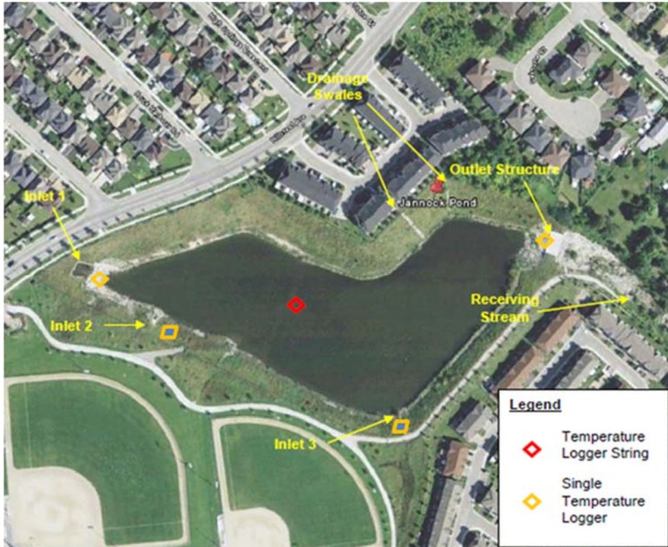
Figure 30: Example of a temperature logger deployment strategy for a pond.
