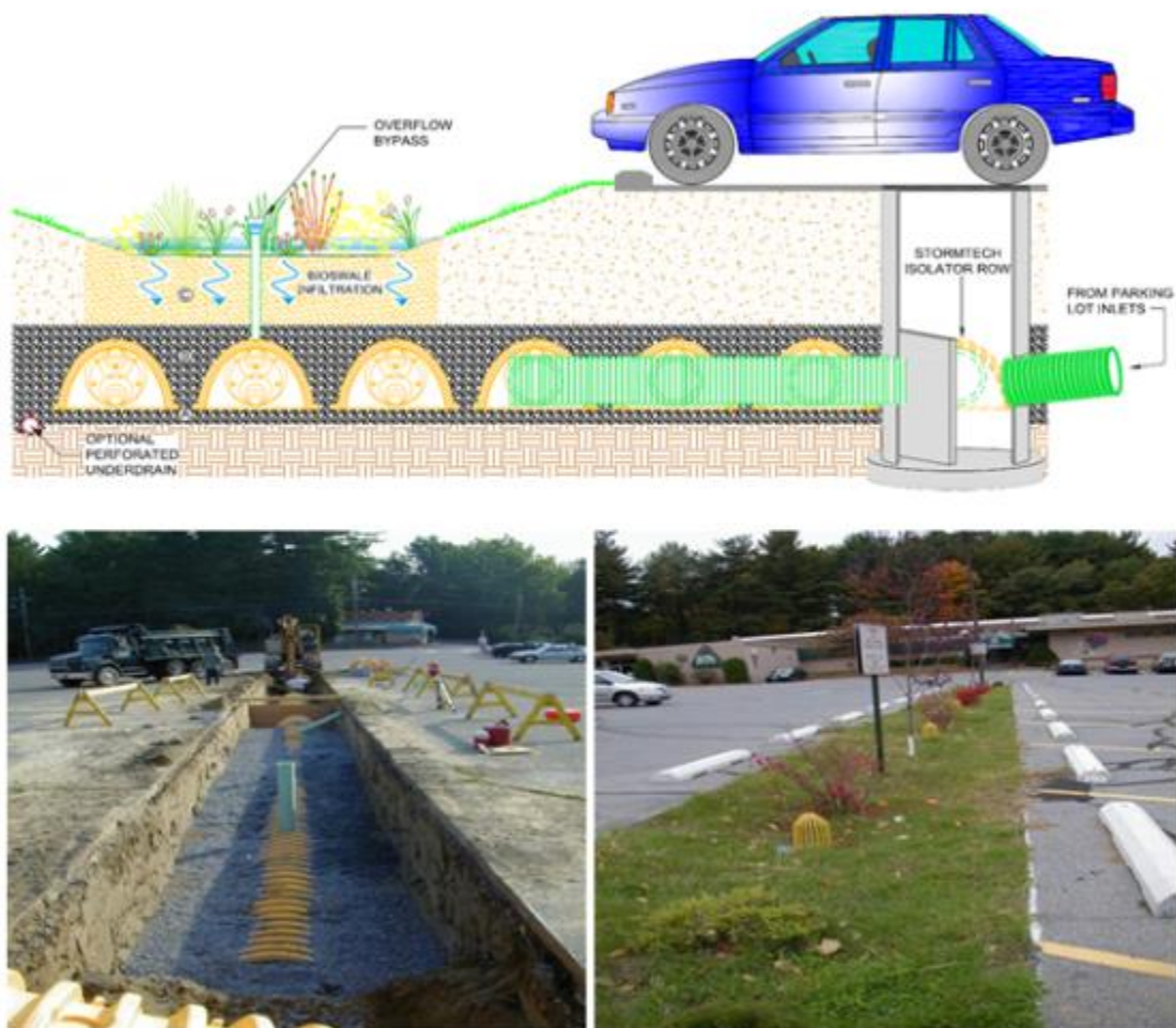
Figure A 8 Examples of large subsurface stormwater storage chambers, which can be incorporated within many pre-existing land use fabrics (Source: ADS Canada).
