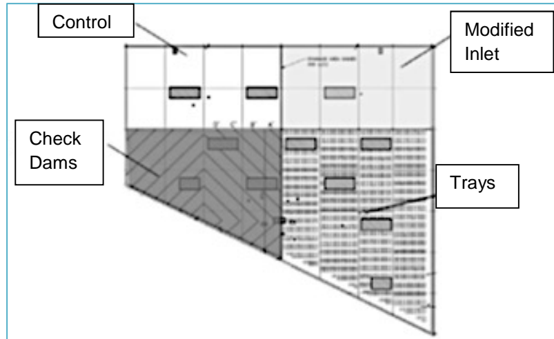
Figure 62: Schematic of roof segments at Metropolitan Avenue pilot Source: NYC Green Infrastructure Plan: 2012 Green Infrastructure Pilot Monitoring Report
