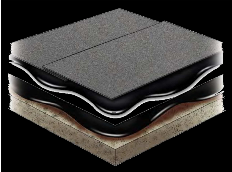
Figure 19: Monolithic Membrane 6125® (American Hydrotech Inc.)
