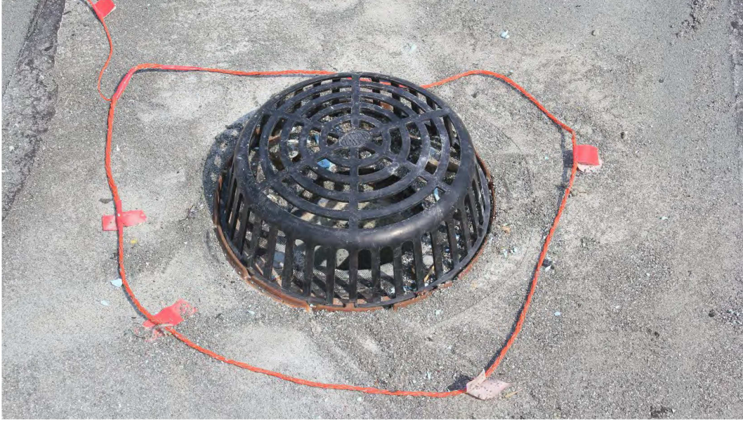
Figure 47: EFVM testing on a roof membrane (American Hydrotech Inc)
