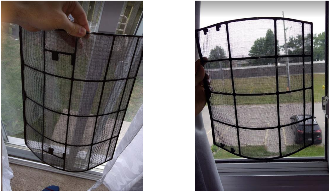
Figure 9-2. The Unit 3 filters showed a minimal amount of dust after 6 months of operation and this is not believed to have impacted the energy savings calculations for this unit.
