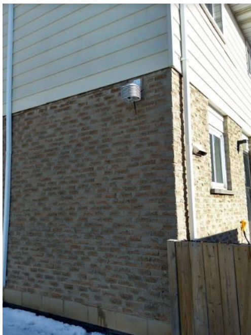
Figure 5-4. An outdoor RH/temperature sensor with radiation shield was installed in the complex.
