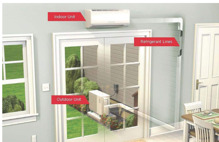
Figure 1-1. Components of a ductless mini-split ASHP.
