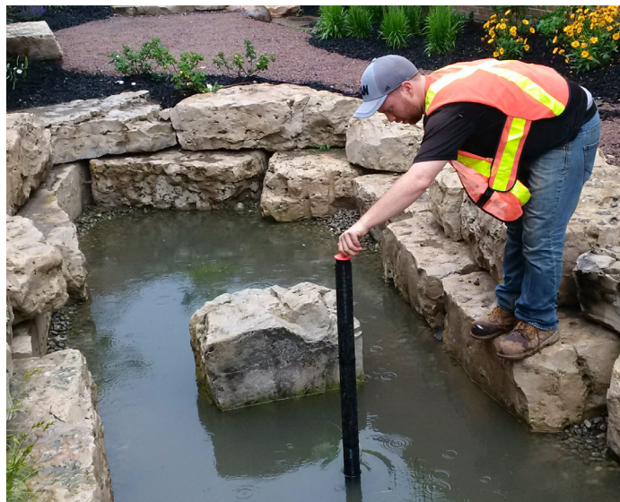
Figure 3. Water level monitoring well being checked
