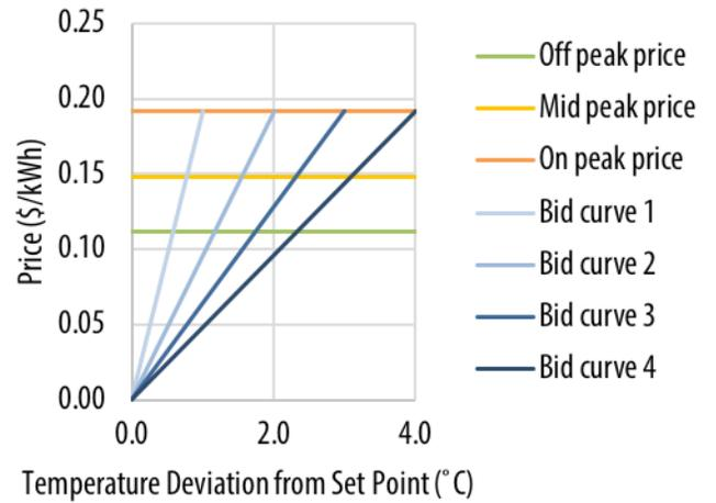
Figure 3. Four example ASHP bid curves compared to variable electricity prices (as of May 2017) used in space heating simulations. From 1 to 4, the curves represent an increasing “willingness to participate”, or a greater threshold for thermal discomfort.
