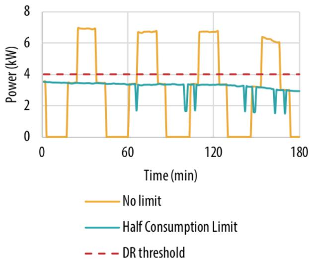
Figure 4. Total simulated ASHP power consumption for a four-house community. Data in yellow indicates transactive control with no demand cap. Data in blue-green shows the response of the system to a DR signal requesting a 50% power reduction. This shows that the transactional system effectively managed the four-house community such that a maximum of two heat pumps would come online at one time, reducing peak loads.
