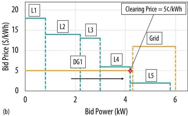
Figure 2. An example of supply and demand curves evaluated in the Energy Marketplace at two consecutive points in time. The bid price of a load (L1 – L5) or supplier (DG1, Grid) is indicated by the height of the respective section of the curves, while the requested or available power is the width of each section of the curves. From (a) to (b) DG generation increases with time, lowering the market clearing price and allowing L4 to power on. Loads can also modify their bids over time.
