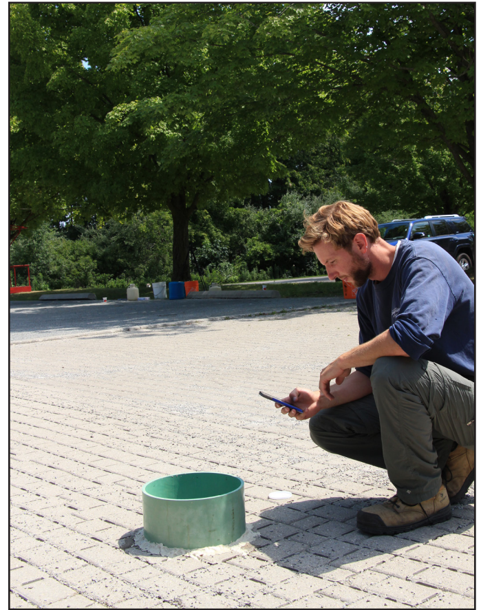
Figure 6. Surface infiltration testing with single-ring infiltrometer
