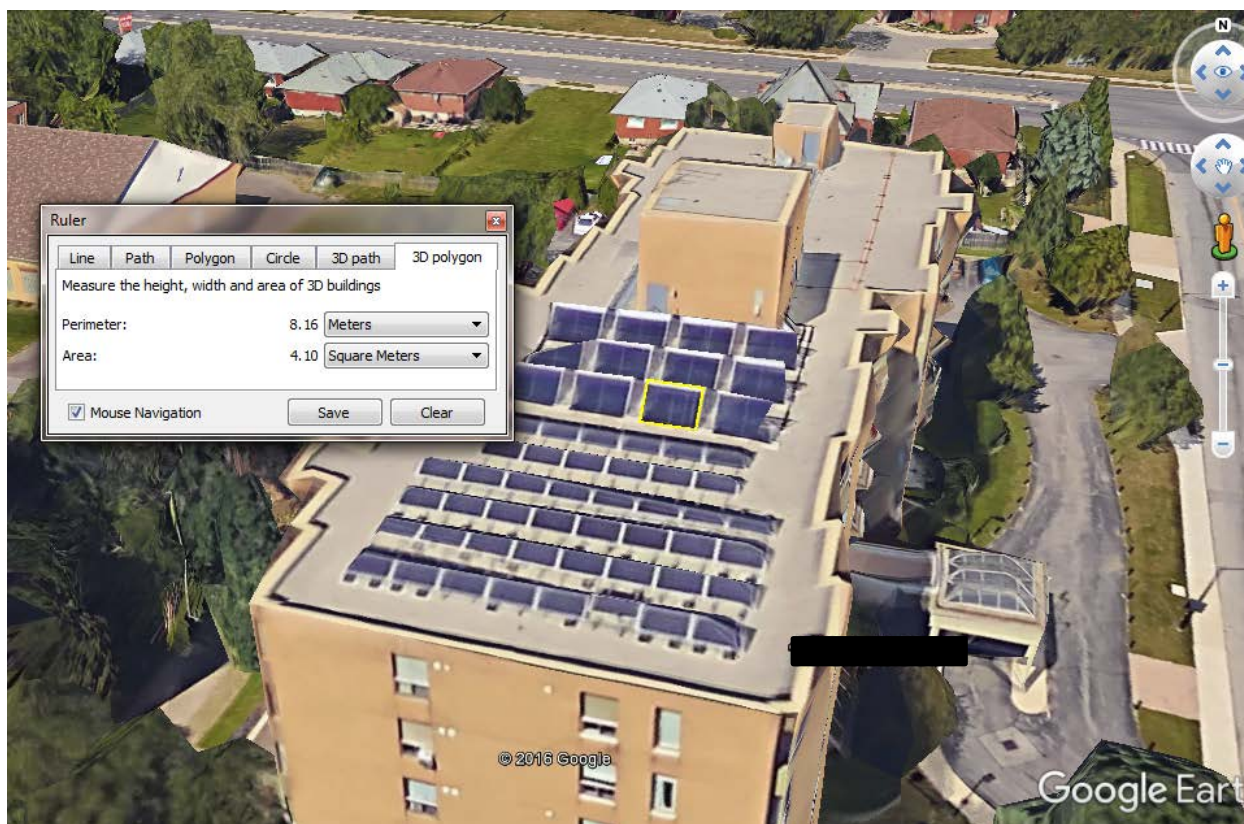
Figure 3-18. Using the estimation procedure outlined in this section, the annual energy produced by the SDHW system a private housing provider's building in Southern Ontario was estimated to be 22,250 [kWh].
