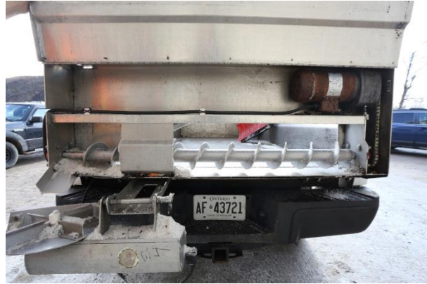
Figure 2. Tailgate spreader showing auger and underside of spinner.
