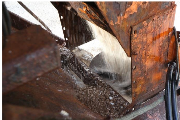
Figure 4. V-box spreader dropping salt onto spinner.
