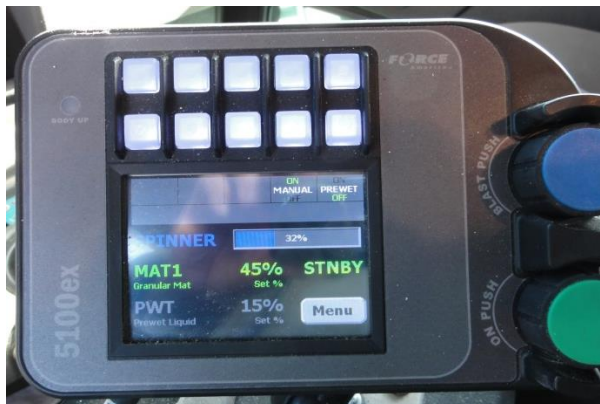
Figure 7. Interface for manual settings of auger and spinner speeds in ground speed controlled spreader (© Robert Roszell 2016).
