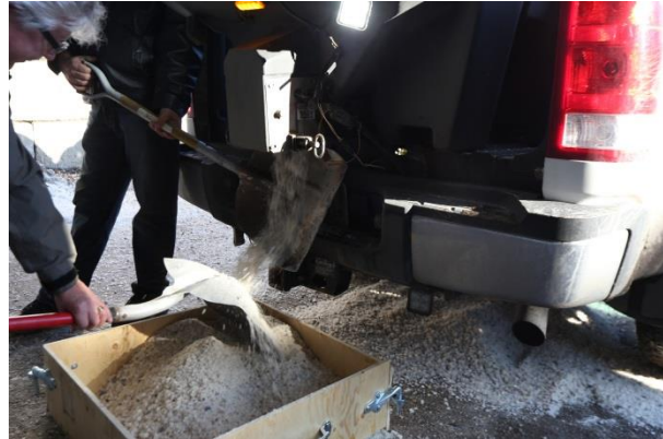
Figure 10. Ensure salt fills evenly into the test box during auger drop test.
