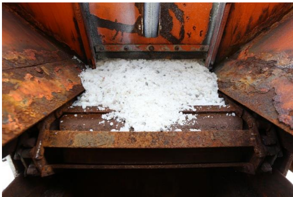
Figure 3. V-box salter gate opening and conveyor belt.
