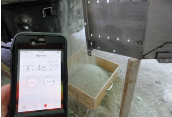
Figure 9. Timing drop test until test box is filled (© Robert Roszell 2016).
