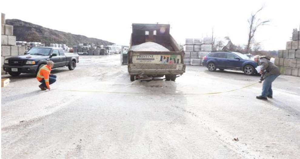
Figure 8. Measurement of the width of salt spread for selected spinner setting.
