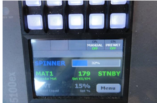
Figure 6. Interface for automatic settings of auger and spinner speeds in ground speed controlled spreader (© Robert Roszell 2016).
