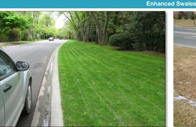
PASS: There is no trash in or around the swale that could possibly block inlets and outlets.
