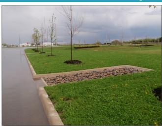
**PASS:** There are no obstructions at the inlet and stormwater can freely flow into the BMP.
