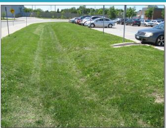
PASS: No erosion gullies or bare soil present at the inlet.
