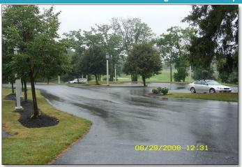
**PASS:** CDA has not changed in size or land cover. Sediment, trash or debris is not accumulating and point sources of contaminants are not visible. (Source: CSN)
