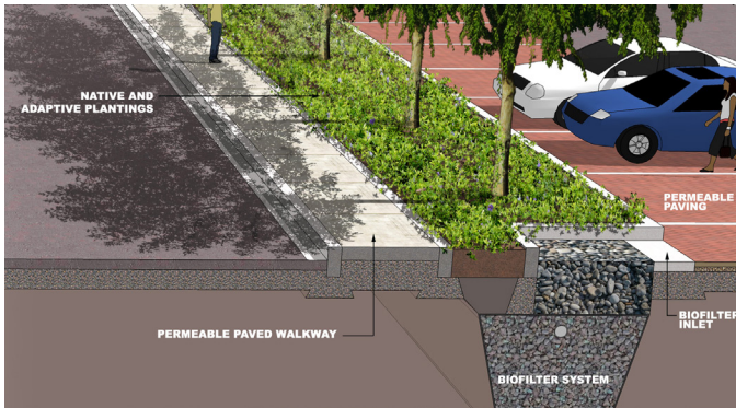
Figure 2. Bifilter design schematic (Image courtesy of Schollen and Company Inc.)
