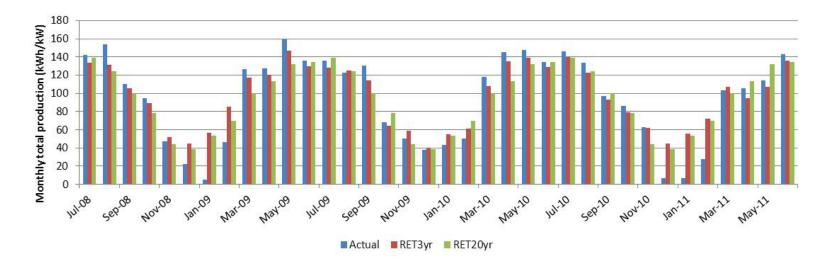
Figure A2. Actual\* vs. RETScreen simulated performance over the 3 year monitoring period.
