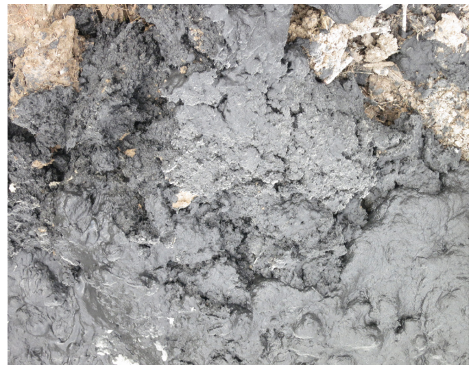
Figure 7. Consistency of sediment after polymer addition.
