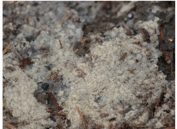
Figure 6. Swelling of LiquiSorb particles following water absorption.
