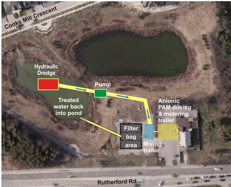
Figure 3. Schematic aerial view of the Pond 4 site during polymer-assisted hydraulic dredging.
