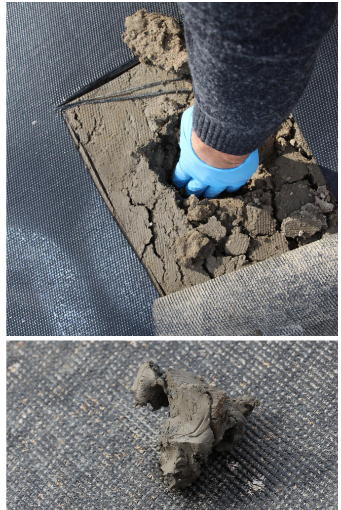
Figure 7. Consistency of Pond 4 sediment at the time of hauling, after two months in the Geotubes™.
