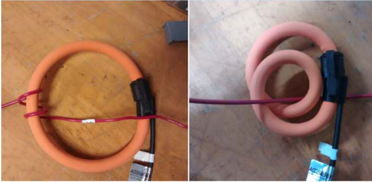
Figure 2.3: The magnitude of the current was increased by either (left) wrapping the wire around the CT or (right) wrapping the CT around the wire.
