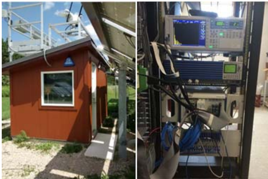
Figure 3.1.3: (Left) A small hut housing PV instrumentation is the primary load on the section of the EPS being monitored for power quality. (Right) The Yokogawa WT1800 is installed on a server rack within the hut.
