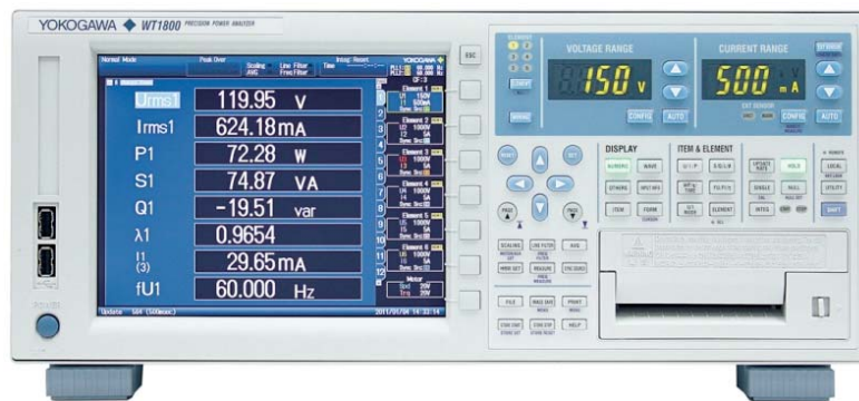
Figure 2.1: The Yokogawa WT180 PQA is a high-end bench-top PQA used in this study.
