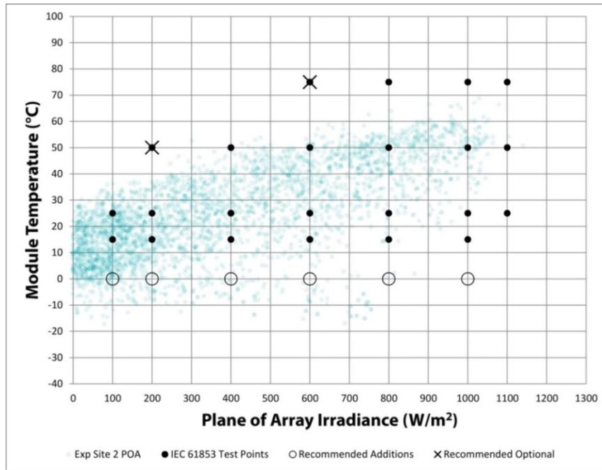
**Figure 3.17** Hourly operating points of module temperature and irradiance for the Toronto, ON experimental location. Each blue circle represents one hour of operation. Closed circles – existing IEC 61853-1 test points; Open circles – proposed new test points; X's – proposed omissions to IEC 61853-1.
