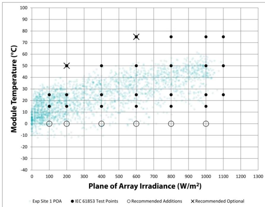
**Figure 3.16.** Hourly operating points of module temperature and irradiance for the St. Catharines, ON experimental location. Each blue circle represents one hour of operation. Closed circles – existing IEC 61853-1 test points; Open circles – proposed new test points; X’s – proposed omissions to IEC 61853-1.
