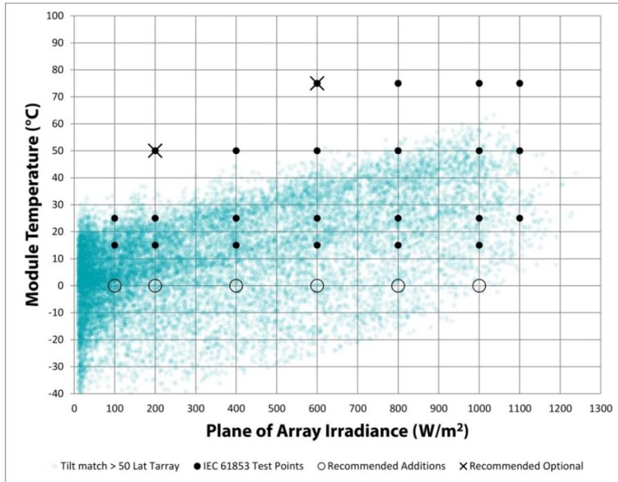
**Figure 3.13.** Frequency of occurrence for operating conditions for latitude match PV installations in Canada. Each blue circle represents one hour of operation. Closed circles – existing IEC 61853-1 test points; Open circles – proposed new test points; X’s – proposed omissions to IEC 61853-1.
