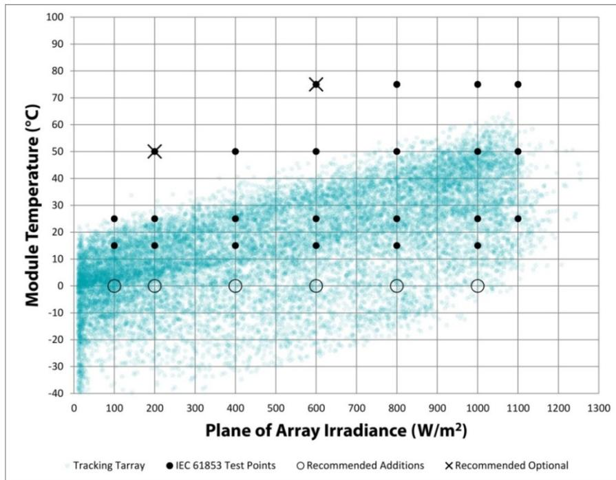
**Figure 3.9.** Frequency of occurrence for operating conditions for dual-tracking PV installations in Canada. Each blue circle represents one hour of operation. Closed circles – existing IEC 61853-1 test points; Open circles – proposed new test points; X's – proposed omissions to IEC 61853-1.
