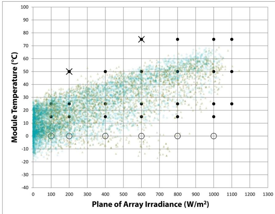
**Figure 2.** Hourly operating points of module temperature and irradiance for the Toronto, ON experimental location (beige triangles) and the Toronto, ON PVsyst modelled location (blue circles). Each circle/triangle represents one hour of operation. Closed circles – existing IEC 61853-1 test points; Open circles – proposed new test points; X’s – proposed omissions to IEC 61853-1.
