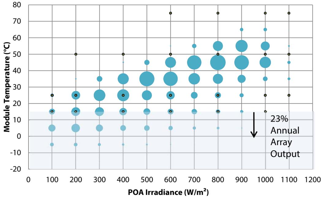
**Figure 3.3.** Array energy output for both ground- and roof- mount configurations for Ontario locations. Bubble area is proportional to the energy output at the given module temperature and irradiance operating point.
