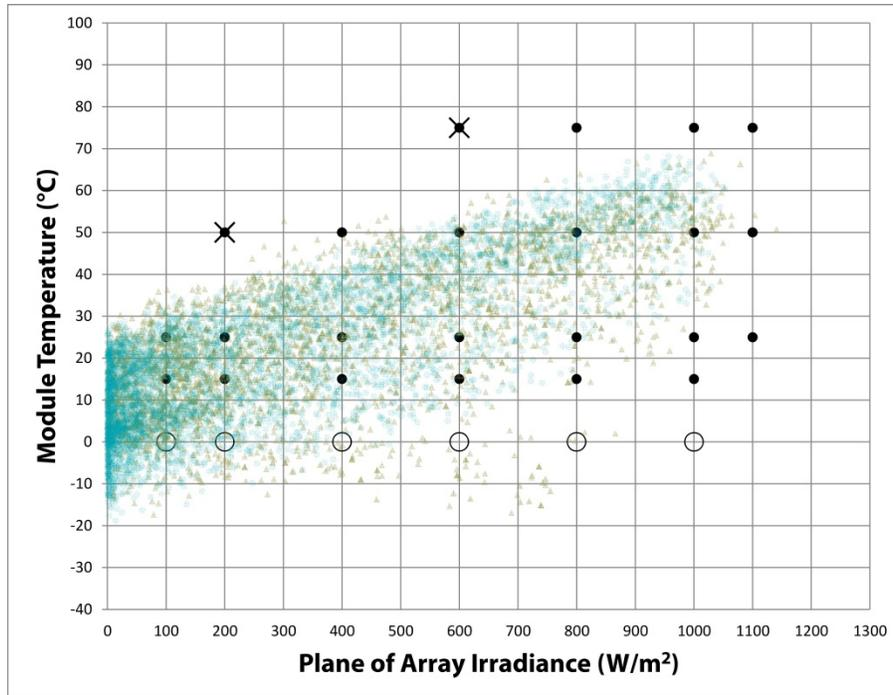
**Figure 3.21.** Hourly operating points of module temperature and irradiance for the Toronto, ON experimental location and the Toronto, ON PVsyst modelled location. Each circle/triangle represents one hour of operation. Closed circles – existing IEC 61853-1 test points; Open circles – proposed new test points; X's – proposed omissions to IEC 61853-1.
