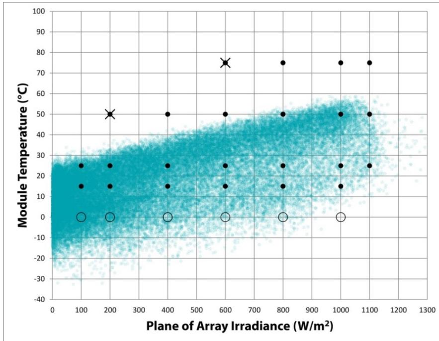
**Figure 3.2.** Module temperature and irradiance operating conditions for ground-mount PV installations in Ontario. Each data point represents one hour of operation. Closed circles – existing IEC 61853-1 test points; Open circles – proposed new test points; X's – proposed omissions to IEC 61853-1.
