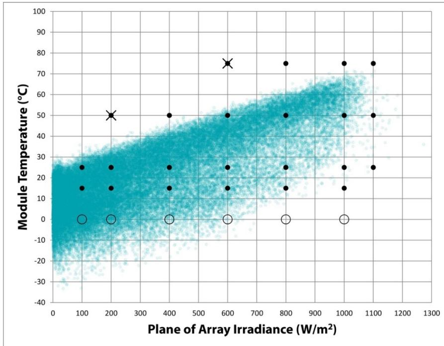
**Figure 3.1.** Module temperature and irradiance operating conditions for roof-mount PV installations in Ontario. Each data point represents one hour of operation. Closed circles – existing IEC 61853-1 test points; Open circles – proposed new test points; X's – proposed omissions to IEC 61853-1.
