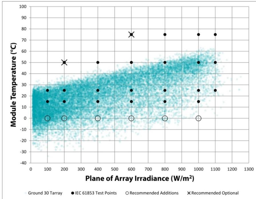
**Figure 3.7.** Frequency of occurrence for operating conditions for ground-mount PV installations in Canada. Each blue circle represents one hour of operation. Closed circles – existing IEC 61853-1 test points; Open circles – proposed new test points; X’s – proposed omissions to IEC 61853-1.
