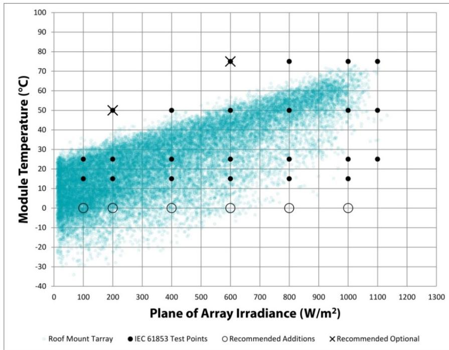
**Figure 3.5.** Frequency of occurrence for operating conditions for roof-mount PV installations in Canada. Each blue circle represents one hour of operation. Closed circles – existing IEC 61853-1 test points; Open circles – proposed new test points; X’s – proposed omissions to IEC 61853-1.
