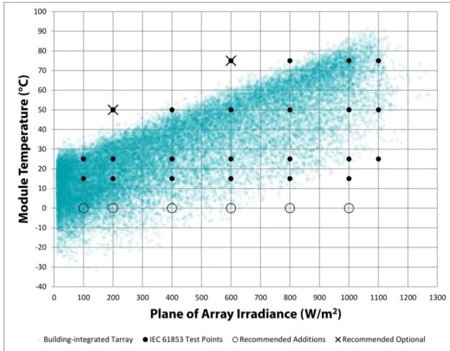
**Figure 3.11** Frequency of occurrence for operating conditions for BIPV installations in Canada. Each blue circle represents one hour of operation. Closed circles – existing IEC 61853-1 test points; Open circles – proposed new test points; X’s – proposed omissions to IEC 61853-1.
