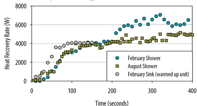
Figure 3. Heat recovery rates for tested events.
