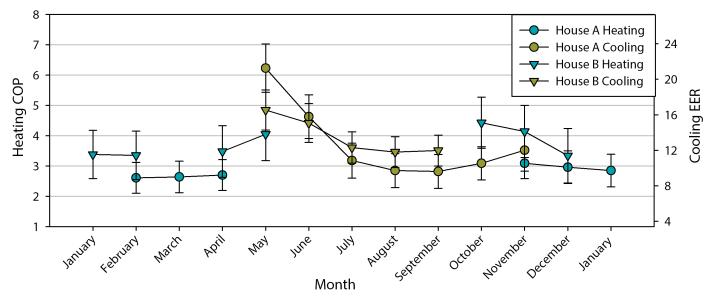
Figure 2. The monthly COP and EER from Peel House A and B.
