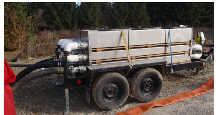
Figure 2: Polymer mixing tank.
