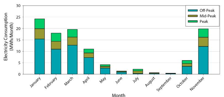
Figure 3. The monthly electrical consumption of the geoexchange system shows that the free-exchange mode of operation is able to cool the building with only minimal electrical energy. Included in this plot is the electricity required for the chiller and the ground-loop circulator pumps.
