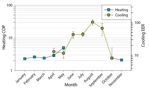
Figure 2. The monthly heating and cooling mode COPs for Earth Rangers. Cooling mode COPs are extremely good due to the primarily free-exchange mode of operation.
