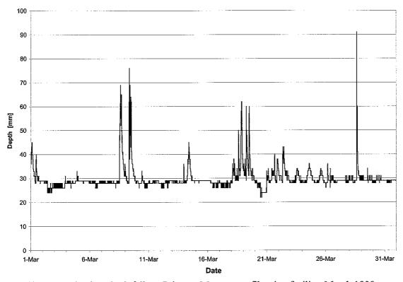
Figure F.12: Water depth and rainfall -- Princess Margaret exfiltration facility, March 1998
