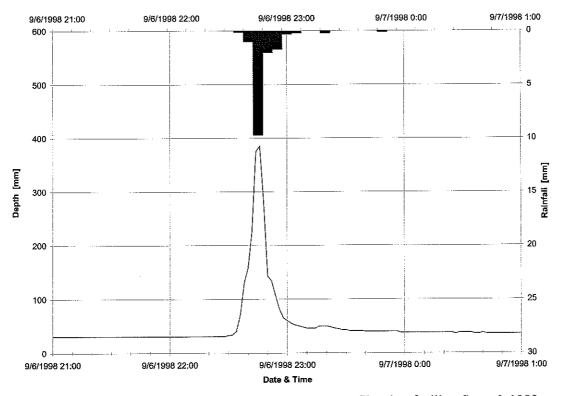
Figure F.22: Water depth and rainfall -- Princess Margaret exfiltration facility, Sept. 6, 1998
