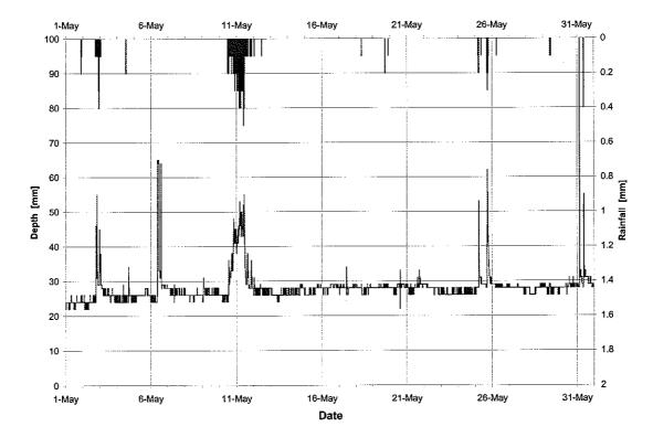
Figure F.14: Water depth and rainfall -- Princess Margaret exfiltration facility, May 1998
