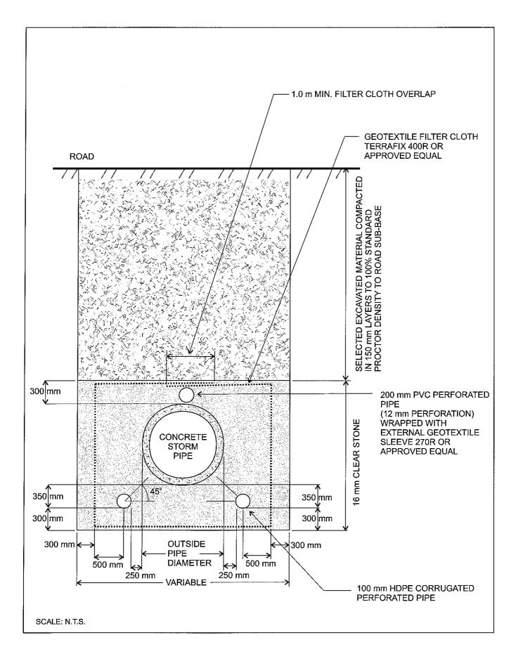
Figure 2.3: Filtration system - typical trench cross-section
