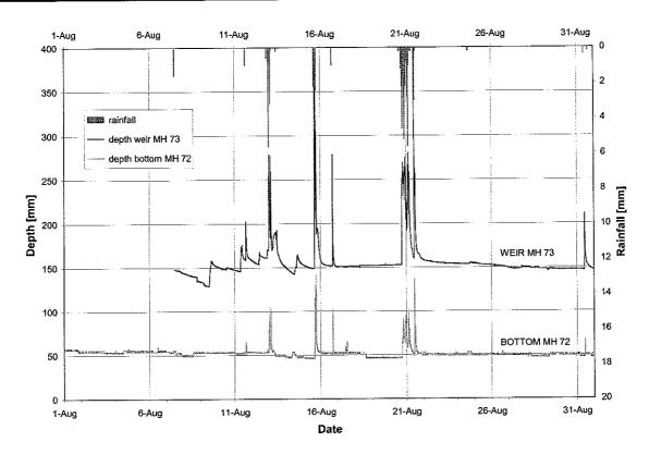
Figure F.5: Water depth and rainfall -- Princess Margaret exfiltration facility, August 1997
