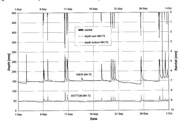
Figure F.6: Water depth and rainfall -- Princess Margaret exfiltration facility, September 1997
