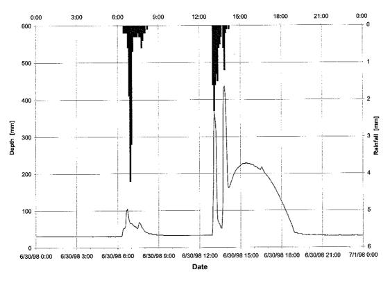
Figure F.21: Water depth and rainfall -- Princess Margaret exfiltration facility, June 30, 1998
