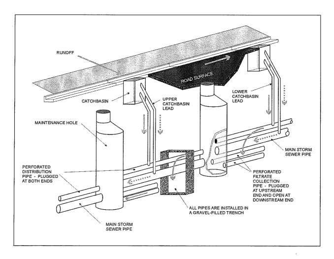
Figure 2: Etobicoke filtration system schematic
