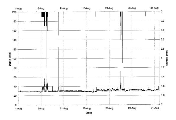
Figure F.17: Water depth and rainfall -- Princess Margaret exfiltration facility, August 1998
