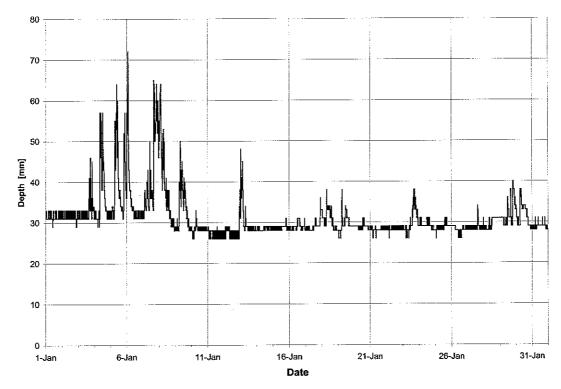
Figure F.10: Water depth and rainfall -- Princess Margaret exfiltration facility, January 1998
