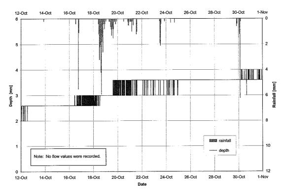
Figure F.1: Water depth and rainfall -- Princess Margaret exfiltration facility, October 1996
