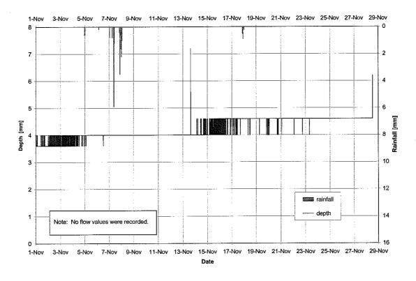
Figure F.2: Water depth and rainfall -- Princess Margaret exfiltration facility, November 1996
