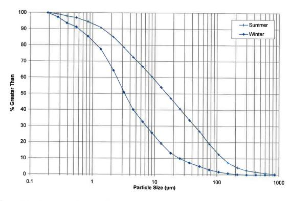
Figure F.25: Average particle size distributions -- Princess Margaret exfiltration facility
