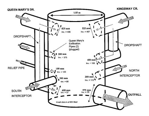
Figure G.5: Schematic diagram of maintenance hole 25
