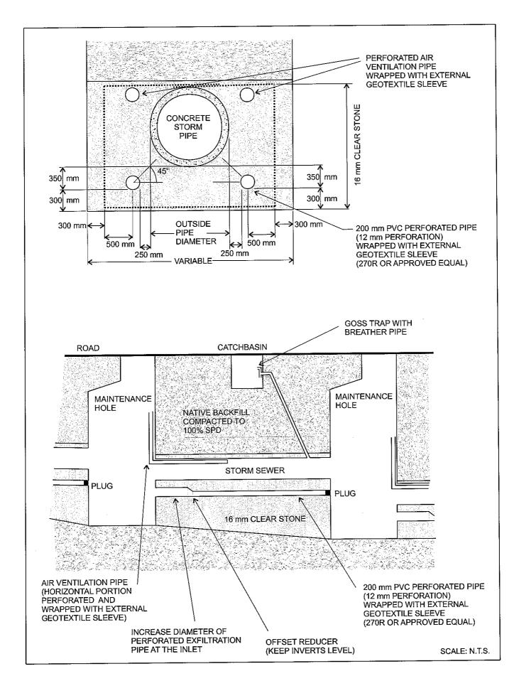
Figure 6.1: Exfiltration system -- suggested revisions
