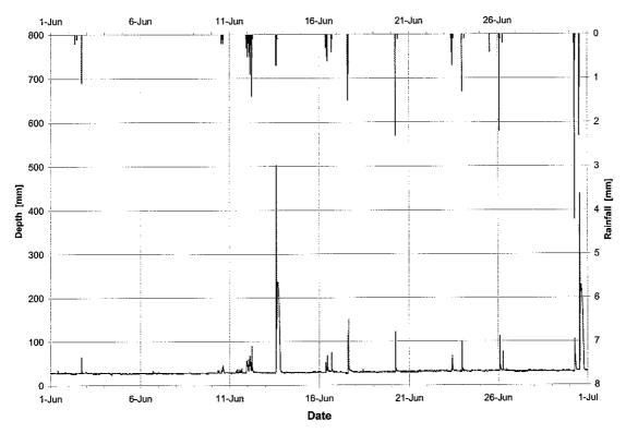
Figure F.15: Water depth and rainfall - Princess Margaret exfiltration facility, June 1998
