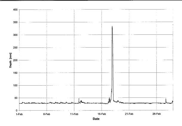
Figure F.11: Water depth and rainfall - Princess Margaret exfiltration facility, February 1998
