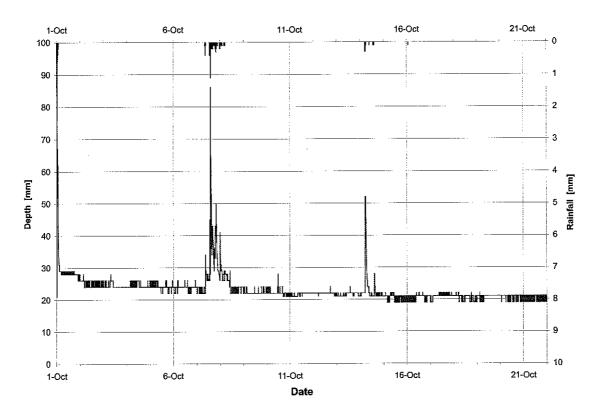
Figure F.19: Water depth and rainfall -- Princess Margaret exfiltration facility, October 1998
