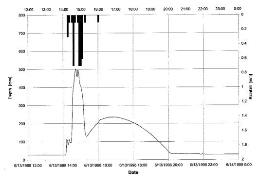
Figure F.20: Water depth and rainfall -- Princess Margaret exfiltration facility, June 13, 1998
