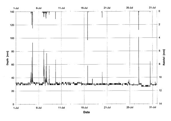
Figure F.16: Water depth and rainfall -- Princess Margaret exfiltration facility, July 1998
