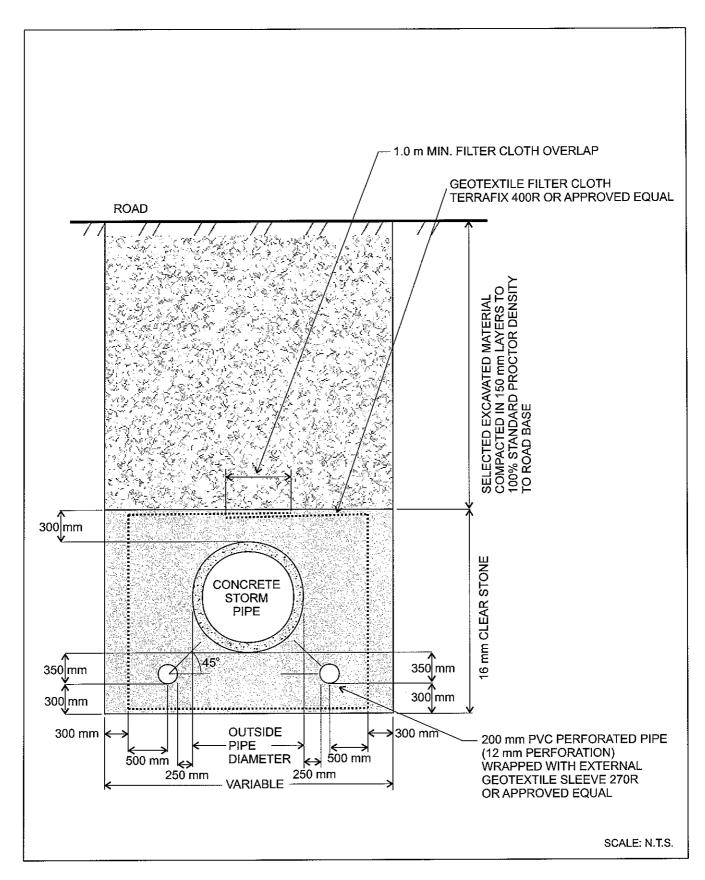
Figure 2.1: Exfiltration system - typical trench cross-section
