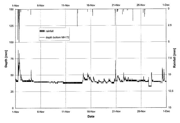
Figure F.8: Water depth and rainfall -- Princess Margaret exfiltration facility, November 1997
