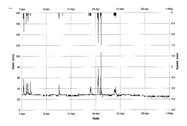
Figure F.13: Water depth and rainfall -- Princess Margaret exfiltration facility, April 1998
