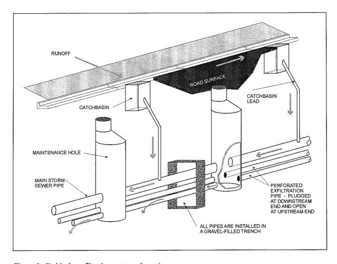
Figure 1: Etobicoke exfiltration system schematic
