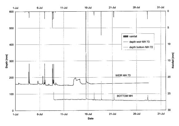
Figure F.4: Water depth and rainfall -- Princess Margaret exfiltration facility, July 1997
