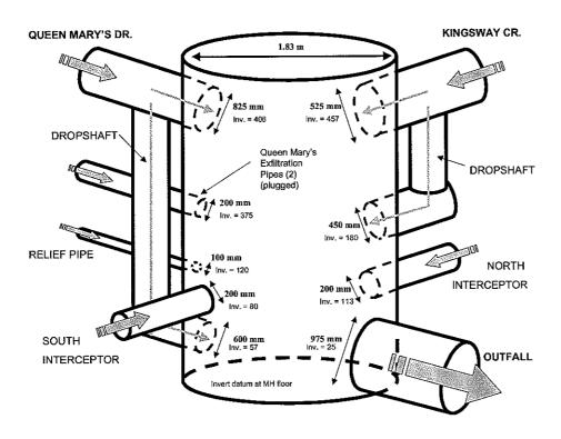
Figure 5.3: Schematic diagram of maintenance hole 25
