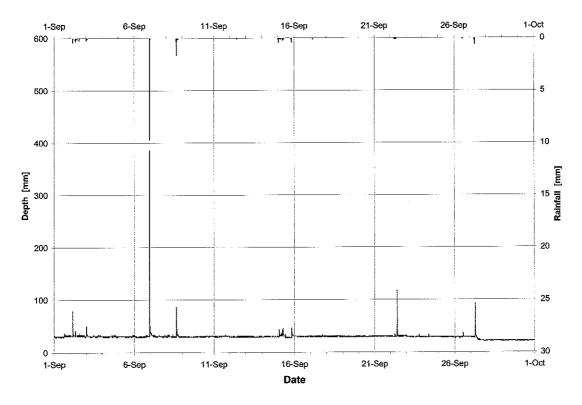
Figure F.18: Water depth and rainfall -- Princess Margaret exfiltration facility, September 1998
