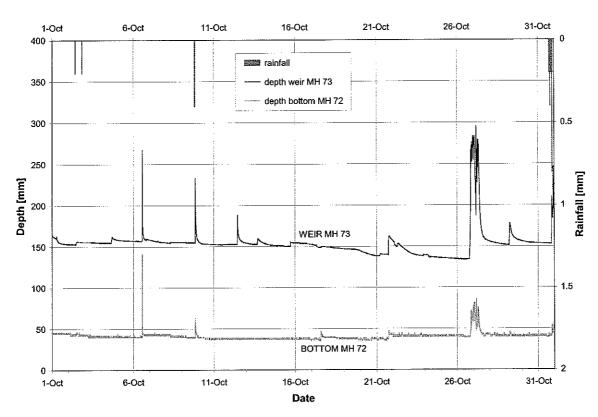
Figure F.7: Water depth and rainfall -- Princess Margaret exfiltration facility, October 1997
