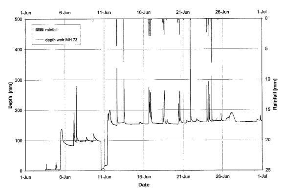
Figure F.3: Water depth and rainfall - Princess Margaret exfiltration facility, June 1997
