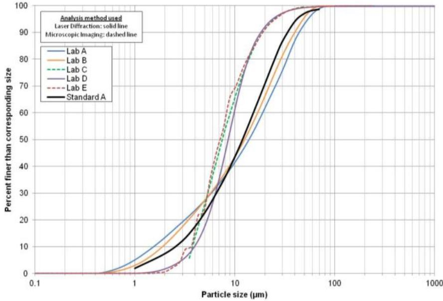
**Figure 4.1:** PSD for test standard and average PSD reported by Labs A, B, C, D and E.
