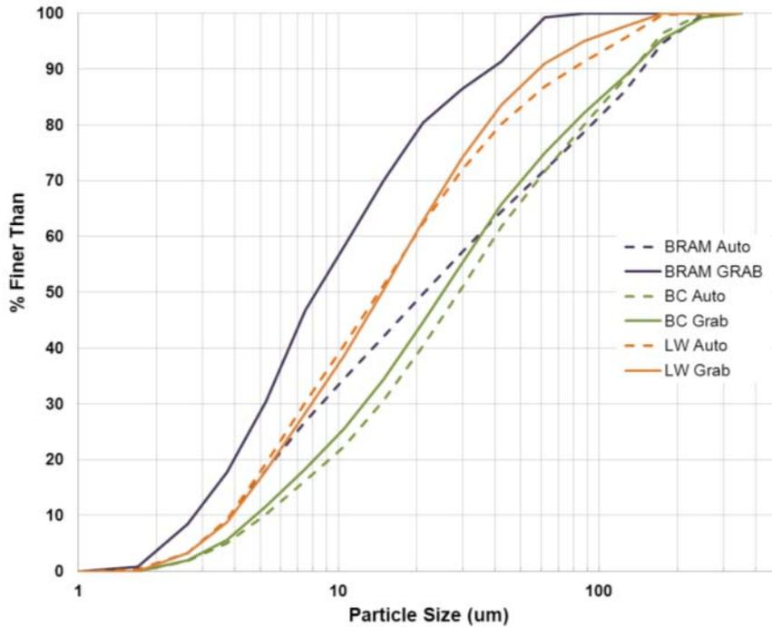
**Figure 5.6:** PSDs of samples collected using an auto sampler or grab method. Samples at the BRAM site were collected at different depths in the water column
