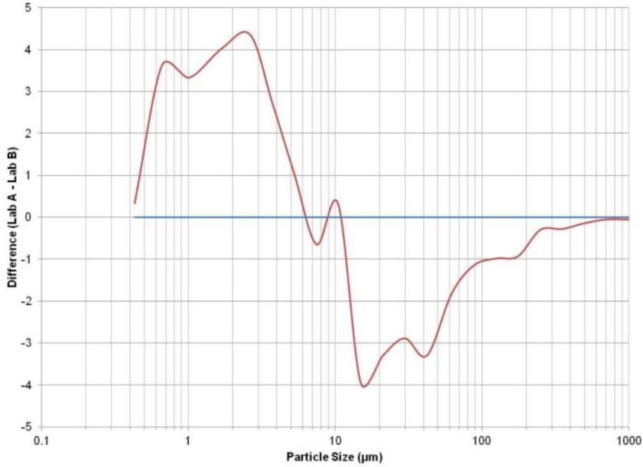
Figure 5.2: Average difference in individual particle size distribution ranges between Lab A and Lab B
