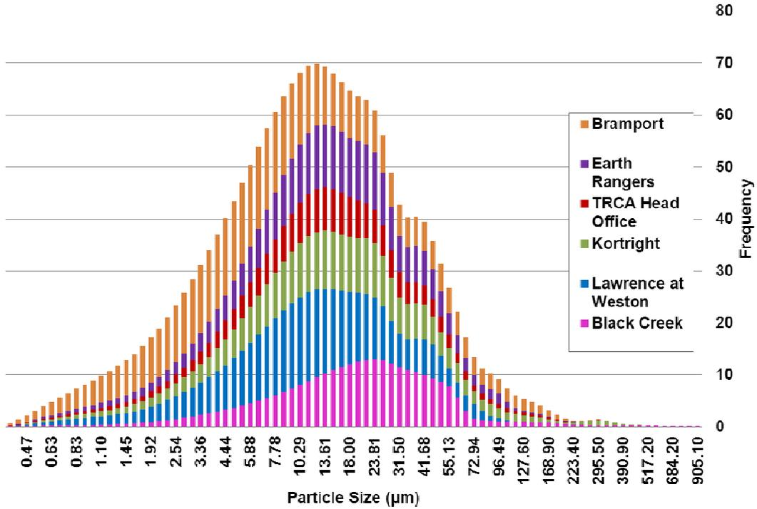
Figure B2: Average PSD for six urban runoff sites in the GTA
