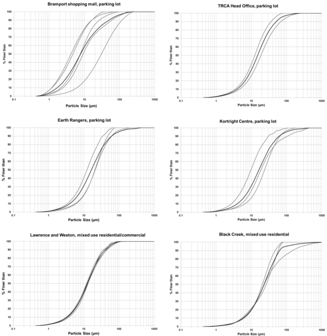
**Figure 5.5:** Average (black) and individual sample (grey) particle size distributions by sampling location
