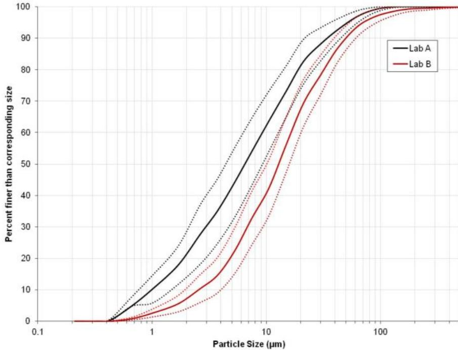
Figure 5.3: Average cumulative PSD for Lab A and B (solid lines) with 95% confidence limits (dotted lines)
