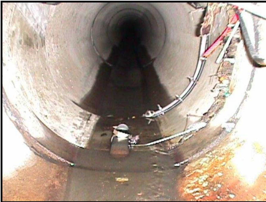
**Figure 4.7:** Area-velocity Probe and Sampling Intake at the Outlet, Stormceptor®
