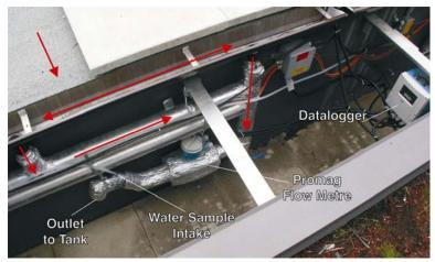
Figure 4.3: Water Quantity and Water Quality sampler set-up
