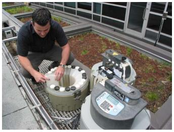
Figure 4.4: ISCO 6700 Water Quality Samplers
