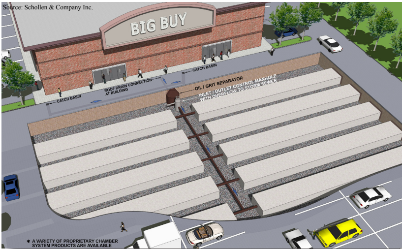
INFILTRATION CHAMBER SYSTEM UNDER A PARKING LOT
