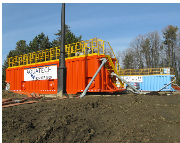
Figure 2.3: TRCA evaluation of an anionic PAM based clarification system using a mixing tank (right) and settling tank (left) installed in series.
