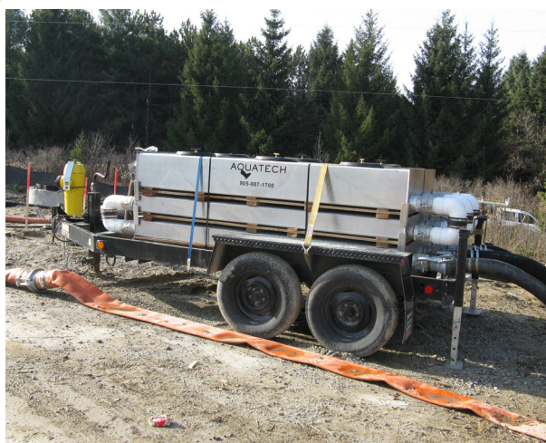
Figure 2.3: TRCA evaluation of an anionic PAM based clarification system using a mixing tank (right) and settling tank (left) installed in series.
