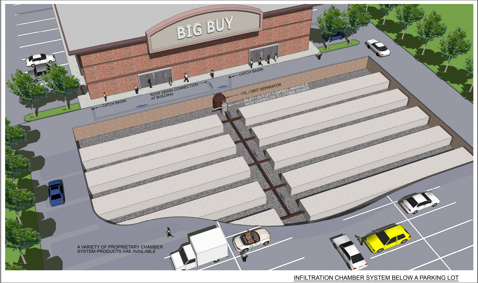
Figure 4.4.7 Schematic of an infiltration chamber system below a parking lot
