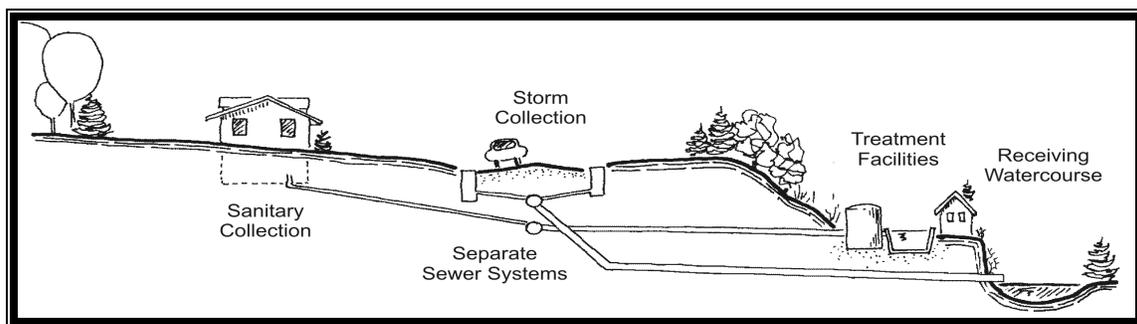
**Figure 2.5 - Separate Collection with Sanitary Treatment**
