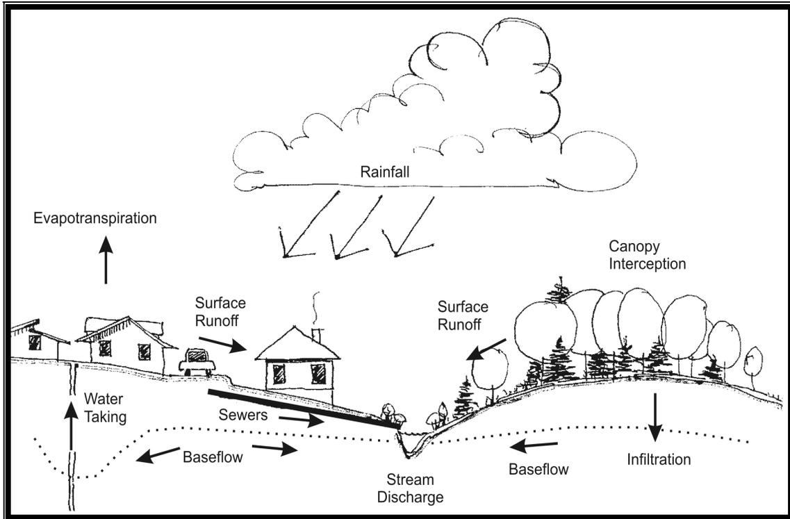
**Figure 2.1 - Hydrologic Cycle Components**
