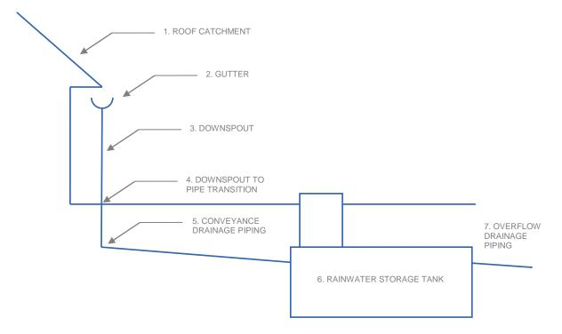
Figure 1-3. Schematic of a typical conveyance network for a below-ground rainwater storage tank
