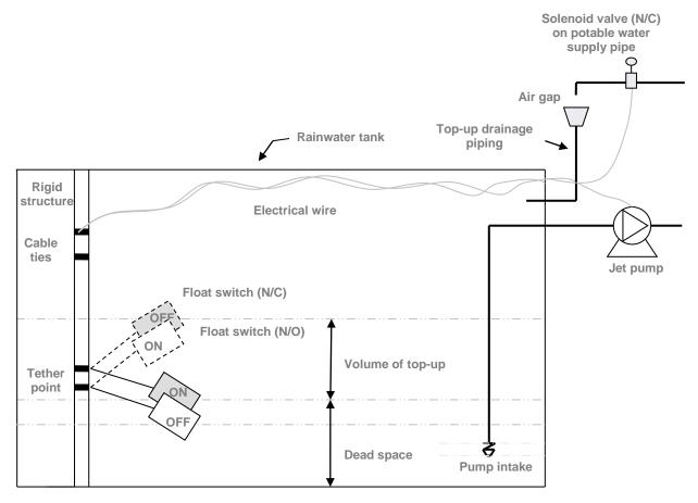
Figure 4-1. Components of an automatic top-up system
