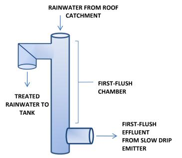
Figure 3-2. Schematic indicating the operation of a first-flush diverter
