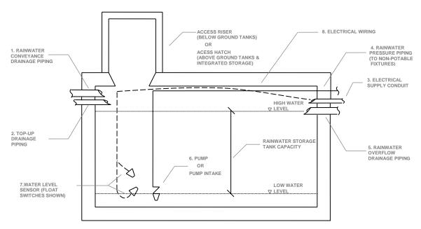
Figure 2-2. Rainwater storage tank schematic
