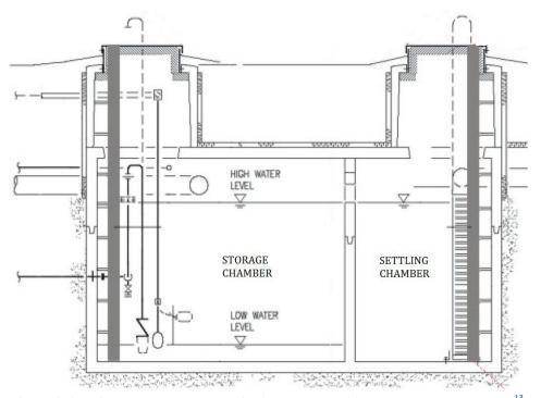
Figure 3-4. Rainwater storage tank with integrated settling and storage chambers 13
