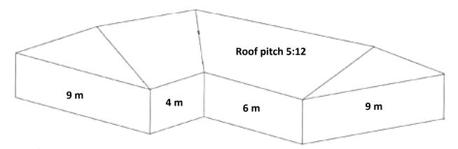
Figure A-1. Roof drainage area to be guttered (isometric 'facing' view)<sup>27</sup>
