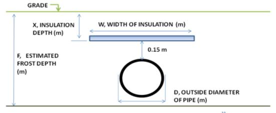
Figure A-5. Frost protection of pipe by horizontal insulation<sup>33</sup>
