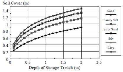
Figure D-3. Soil cover for soakaway pits, based on frost heave<sup>55</sup>
