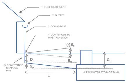
Figure A-4. Pipe conveyance (profile view)
