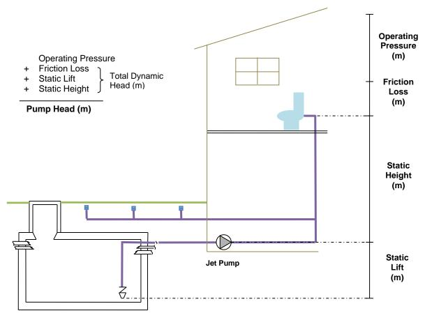
Figure 5-2. Components of Total Dynamic Head (TDH)
