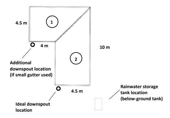
Figure A-2. Roof drainage area to be guttered (projected 'top-down' view)<sup>28</sup>
