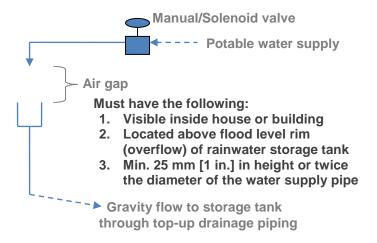
Figure 4-2. Schematic drawing of a top-up system with an air gap<sup>19</sup>
