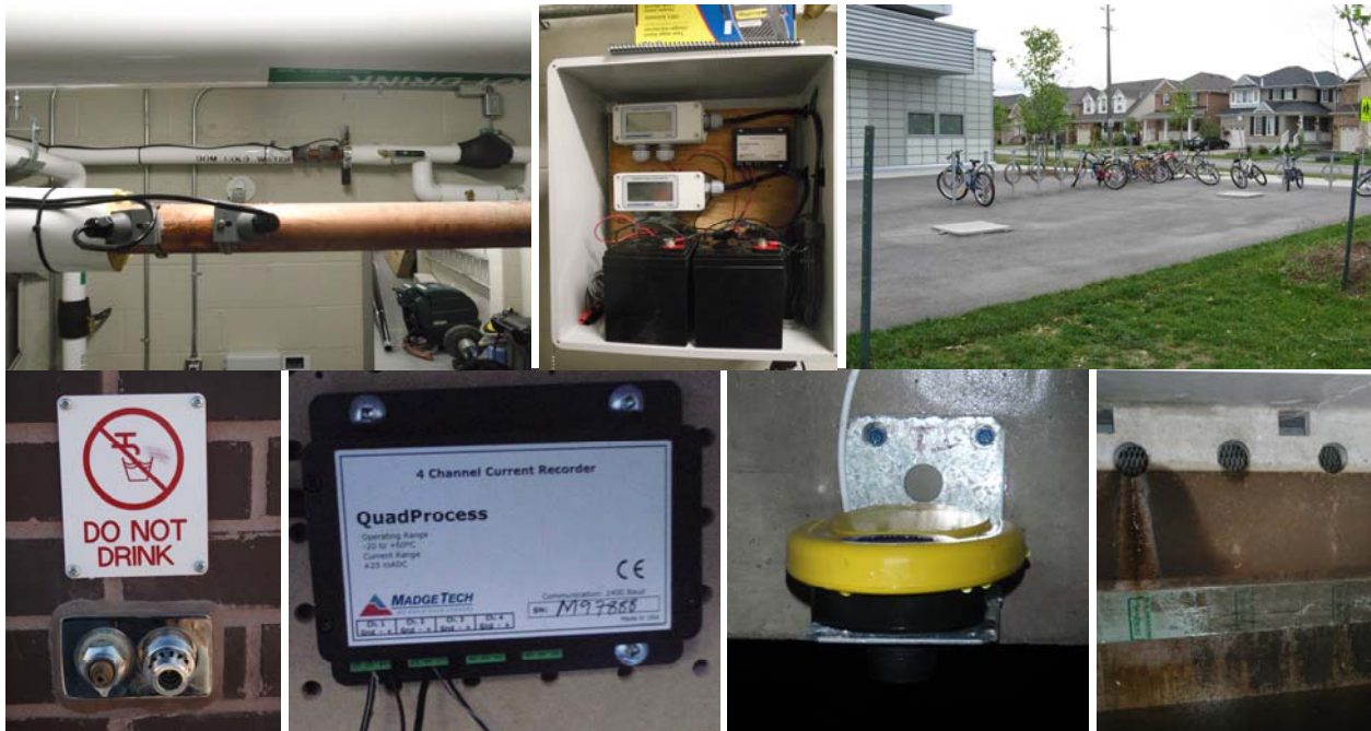
Figure 4.7: Brookside public school monitoring equipment. Clockwise starting from upper left- ultrasonic clamp-on flow meters; flow logger; ground level view of cistern access points; weir inside cistern; ultrasonic level sensor in storage chamber, data logger for ultrasonic level sensors; outside hose bib used for irrigation.
