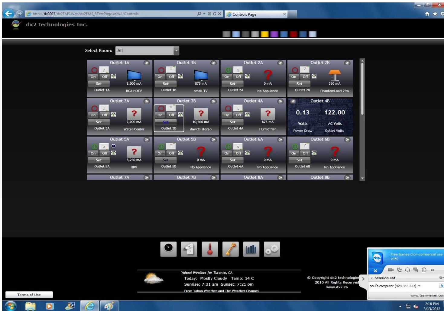
Figure 2.2: The dx2 system control interface for setting up individual appliance control. Each square shows the listed appliance, a receptacle ID, a manual on/off switch, a small arrow on the top right corner that will flip the square to show real time consumption from the individual appliance, and a set button that takes the user to a full screen of control options for the individual appliance.
