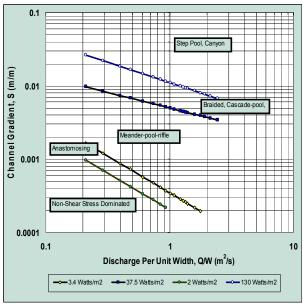
Fig. 6. Specific Stream Power Criteria for Stream Classification (Modified after Brookes 1985) Based on Channels in Southern California and Southern Ontario
