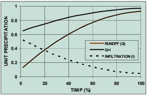
Fig. 1. Change in Hydrologic Budget Parameters (Marsalek, 1991). The increase in runoff volume coupled with improvements in drainage efficiency translates into an increase in the frequency and magnitude of peak flows to the receiving channel for the entire spectrum of flow events experienced by the watercourse (Leopold, 1967). The impact on the hydrologic regime is non-uniform.
