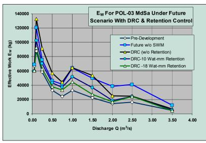
Fig. 4. Particle mobility for medium sand (MdSa assuming a "duration standard" based on the mean particle size fraction ( $\phi_{50} = 35 \text{ mm}$  (minimum range for coarse gravel)) and selected SWM alternatives (Cover et al., 2006). Note that SWM refers to Stormwater Management, DRC is the acronym for Distributed Runoff Control, Wattmm Retention represents the volume of runoff measured in millimetres spread uniformly over the area of the watershed assigned to retention using Source Control.
