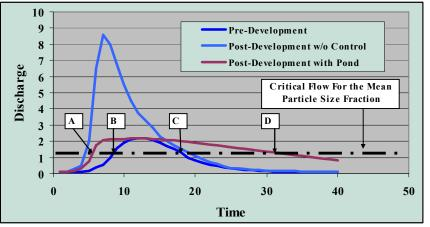
Fig. 3. Illustration of the Effect of Pond Routing On The Post-Development Hydrograph in Comparison With the Pre-Development Hydrograph and the Critical Flow Based on the Mean Particle Size Fraction. Note that the period for which the pre-development flows exceed the critical flow is between points B and C. Following implementation of the Pond this period increases to points A and D with a proportionate increase in the ability of the watercourse to perform work.
