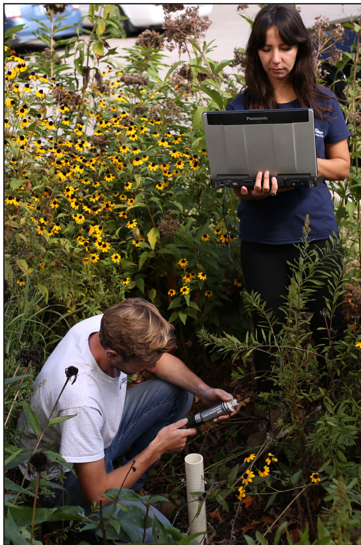
Figure 6. Continuous water level monitoring in a bioretention
